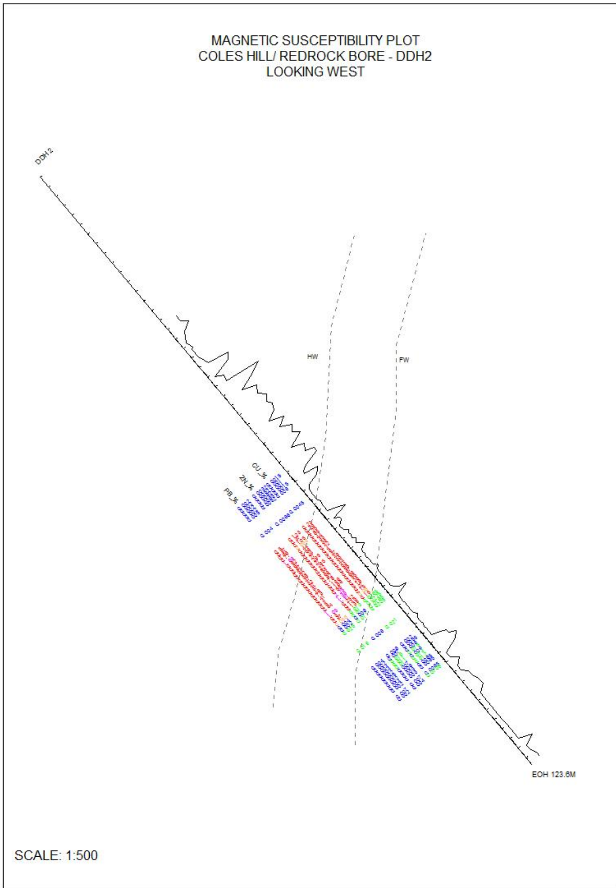
Figure 2: DDH2 – Coles Hill Prospect. Plot of magnetic susceptibility with respect to mineralisation
