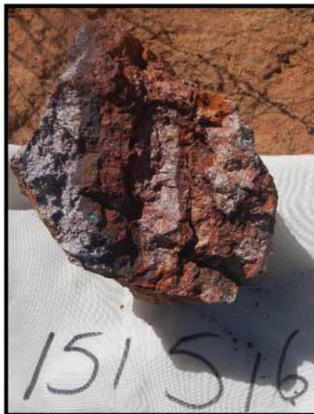
Plate 6. Rock sample 151516. Outcrop in creek bed. Metasediment with Fe-oxide fractures 1mm-1cm wide.
