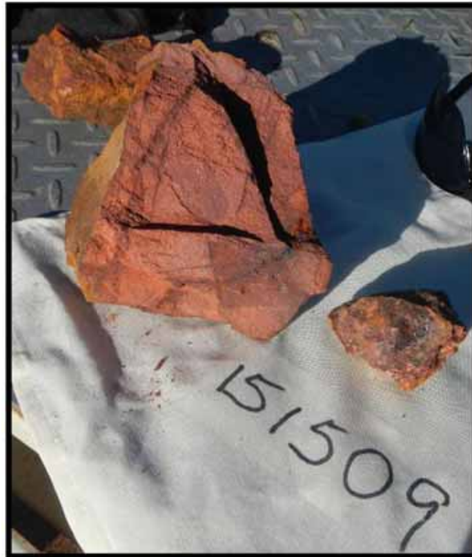
Plate 1. Rock sample 151509. Fine to medium grained greywacke (SSW) with 1-3mm wide haematite fractures throughout. The rock contains a weak penetrative deformation fabric throughout, with minor phyllosilicates developed. Probable Murphy Metamorphics.
