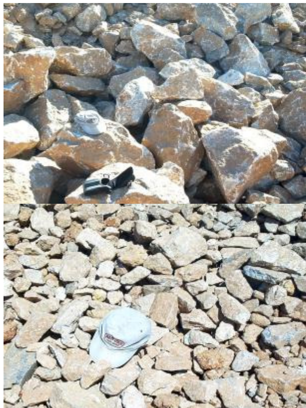
Figure 3. Stockpiles +200mm (top photo) + 10mm (lower photo) of crushed product ready for CML shipment to Norsk Hydro in 1995
