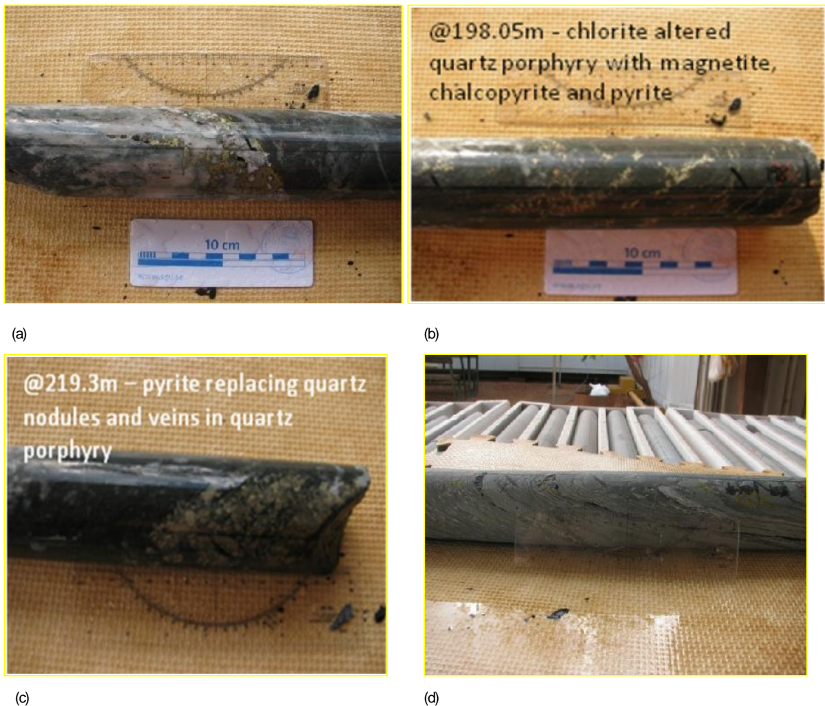
Figure 28: Core photos of CBDD003. (a) 192.85m – quartz vein with chalcopyrite and pyrite in contact with magnetite; (b) 198.05m - chlorite altered quartz porphyry with magnetite, chalcopyrite and pyrite; (c) 219.3m – pyrite replacing quartz nodules and veins in quartz porphyry; (d) 221.7m – strongly foliated quartz porphyry.
