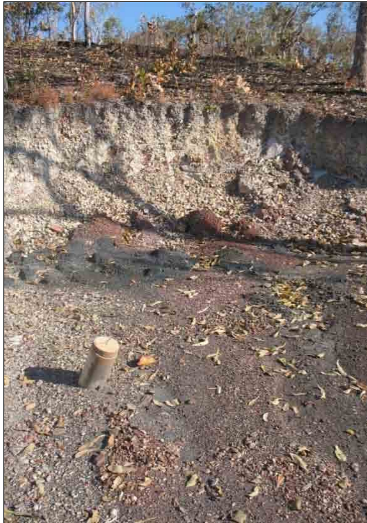
Figure 4 Plugged PVC Collar at MHRC 014
