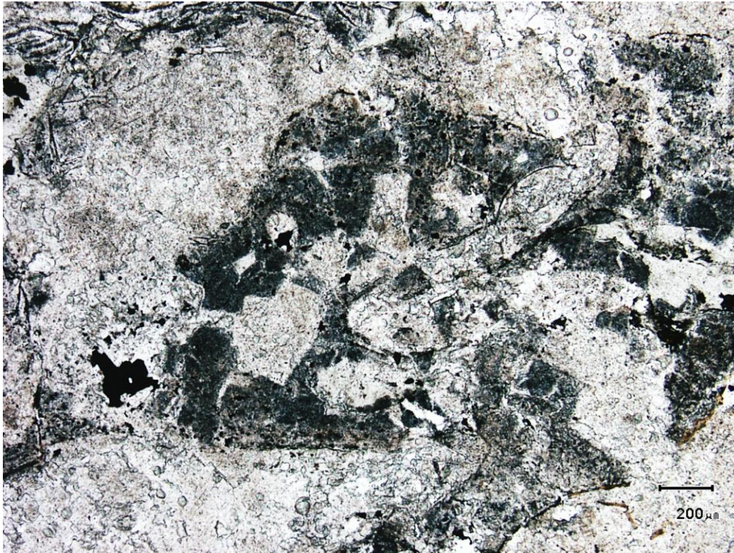
Fig 14 KORC-008, 105m 200 μm TS. PPL. (x50). A dark, oxide-clouded volcanic clast with pale relict phenocrysts, all within carbonate in altered possible lithic-vitric tuff.
