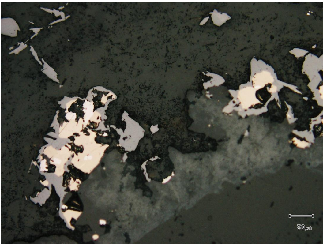
Fig 16 KORC-008, 105m PTS. RPL. (x200). Pale brown pyrrhotite and white pyrite accompanied by grey rutile.
