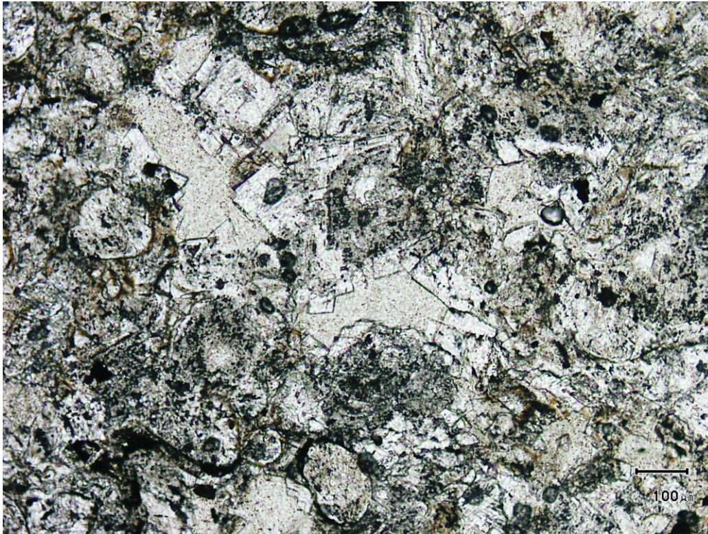
Fig 1 KORCH-007, 52m 100 μm TS. PPL. (x100). Zoned rhombohedral carbonate crystals with interstitial chlorite in massive altered mafic material.
