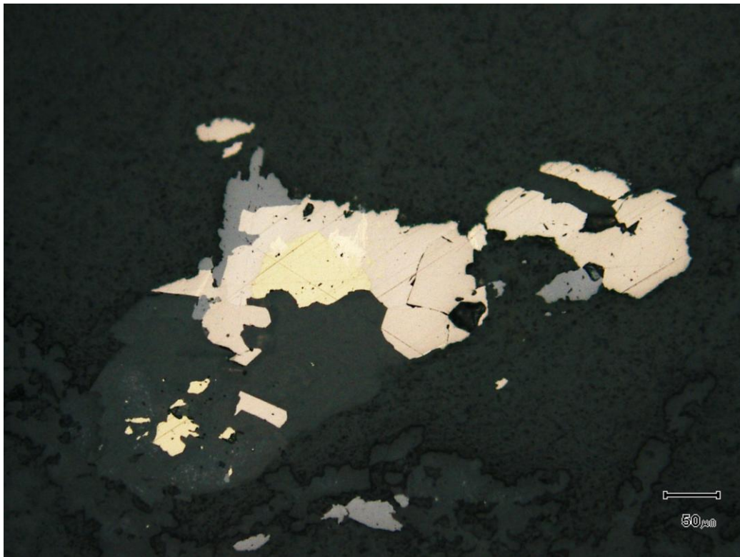
Fig 20 KORCH-008, 115m 50 µm PTS. RPL. (x200). Composite of pyrrhotite, rutile, chalcopyrite, pyrite and sparse finer pentlandite.
