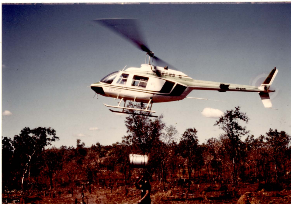
Plate 1-2. Bell 206-B Jet Ranger III helicopter slinging 200 litre (44 Imperial gallons) fuel drums of diesel fuel to drill rig. This helicopter was also utilized for geological fieldwork.
