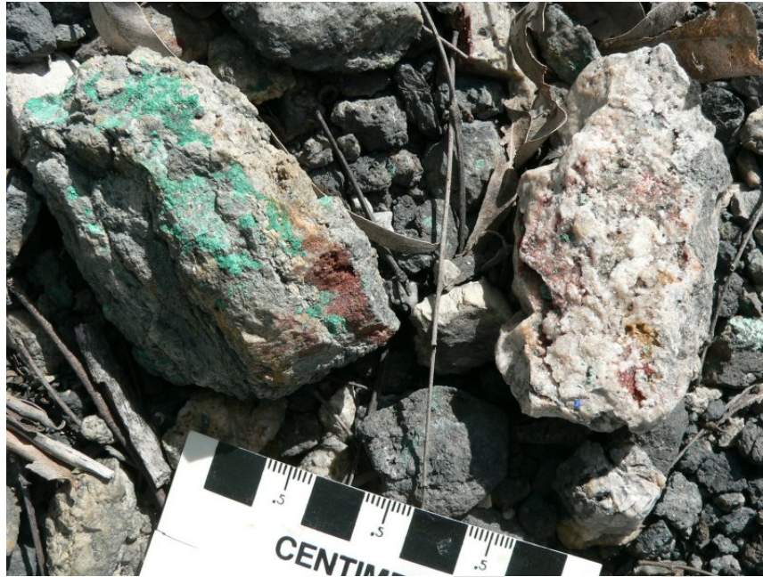
Fig 6 Full Hand – secondary Cu mineralisation, carbonaceous shear, quartz vein
