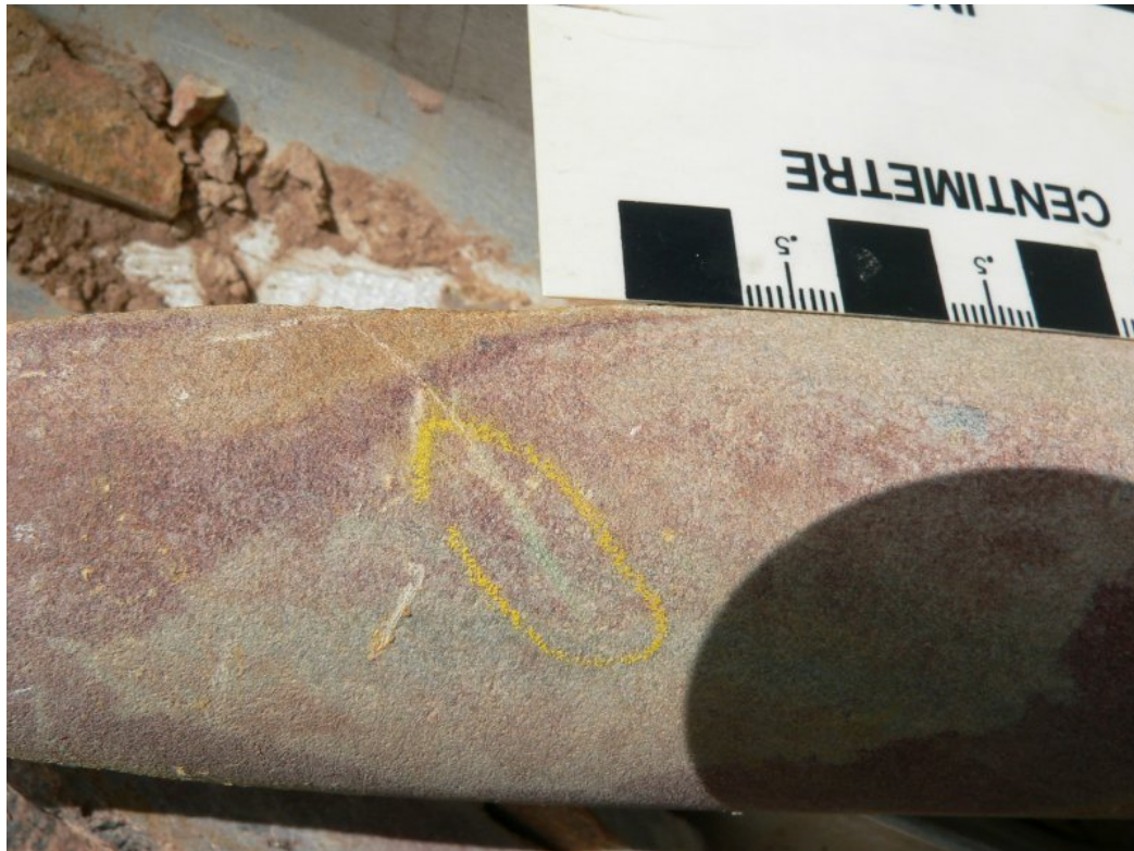
Fig 3 Liberator - secondary U in fracture
