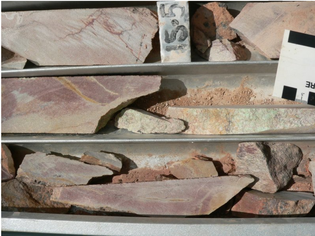
Fig 2 Liberator - secondary U in fractures
