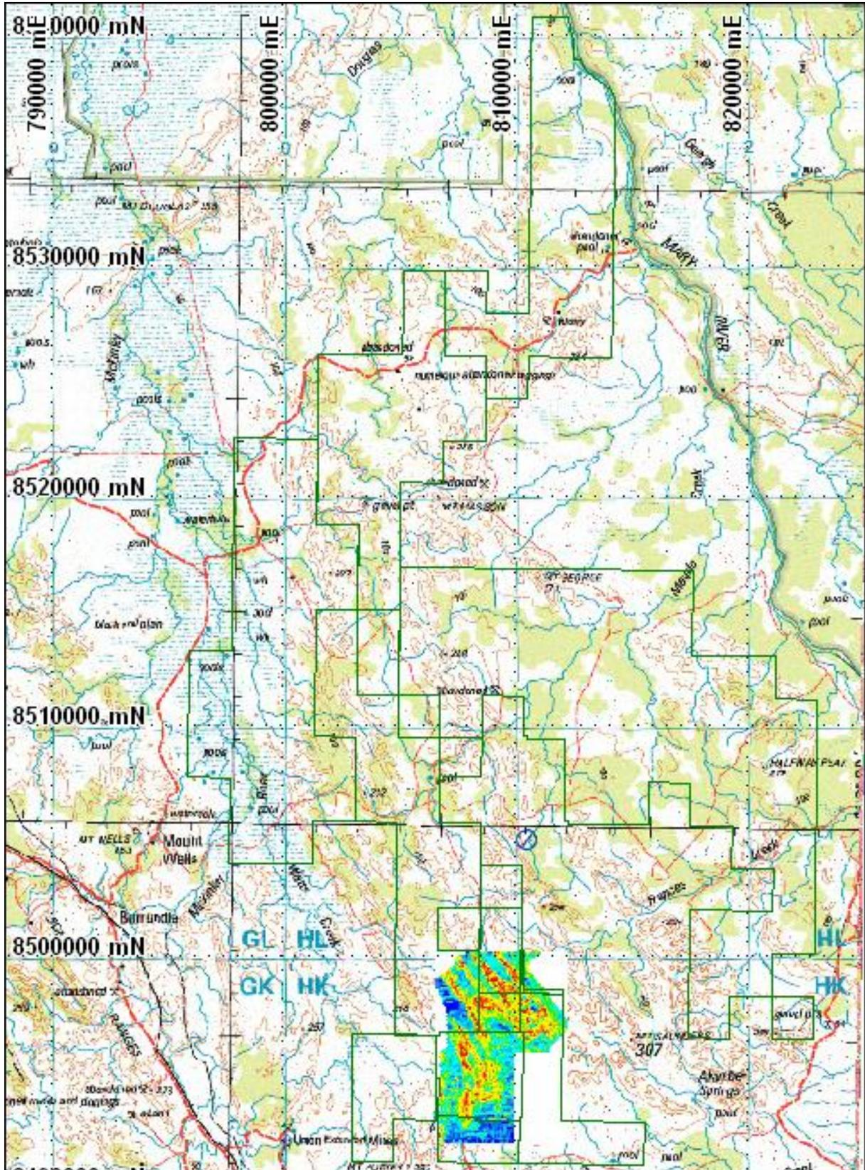
Figure 5: Maximum conductivity response image from the Frances Creek RepTEM survey.
