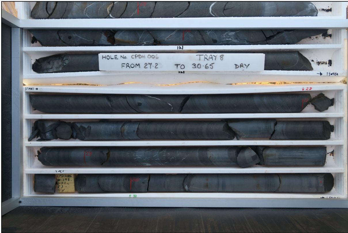
Figure 3 - Hole CPDH006, Lynott Formation, laminated pyrite in carbonaceous siltstone
