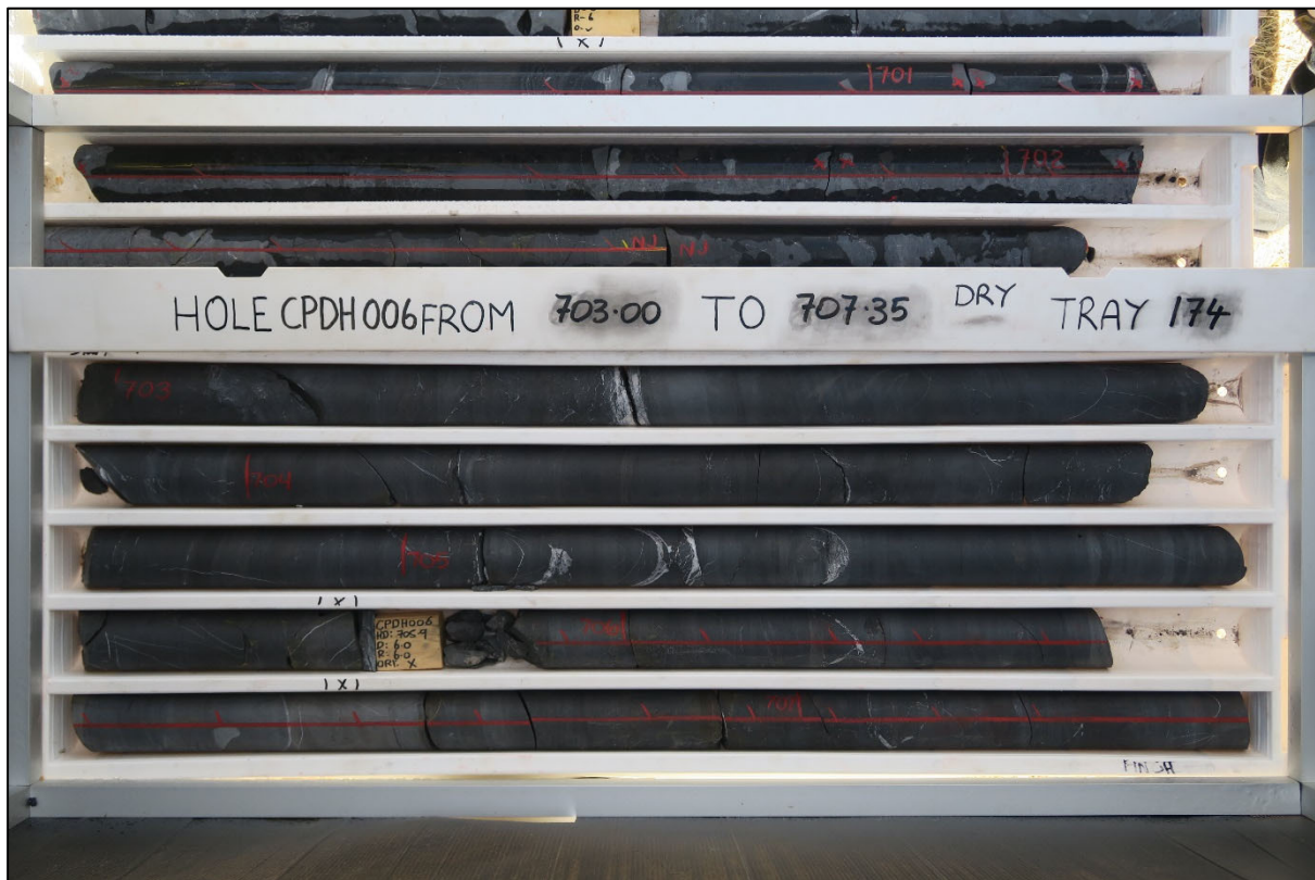
Figure 5 - Hole CPDH006, Barney Creek Formation, sulphidic carbonaceous siltstone
