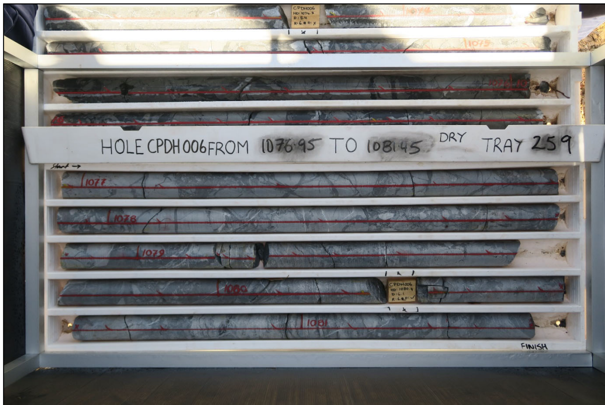
Figure 6 - Hole CODH006, Cooley Dolostone Member, brecciated dolostone
