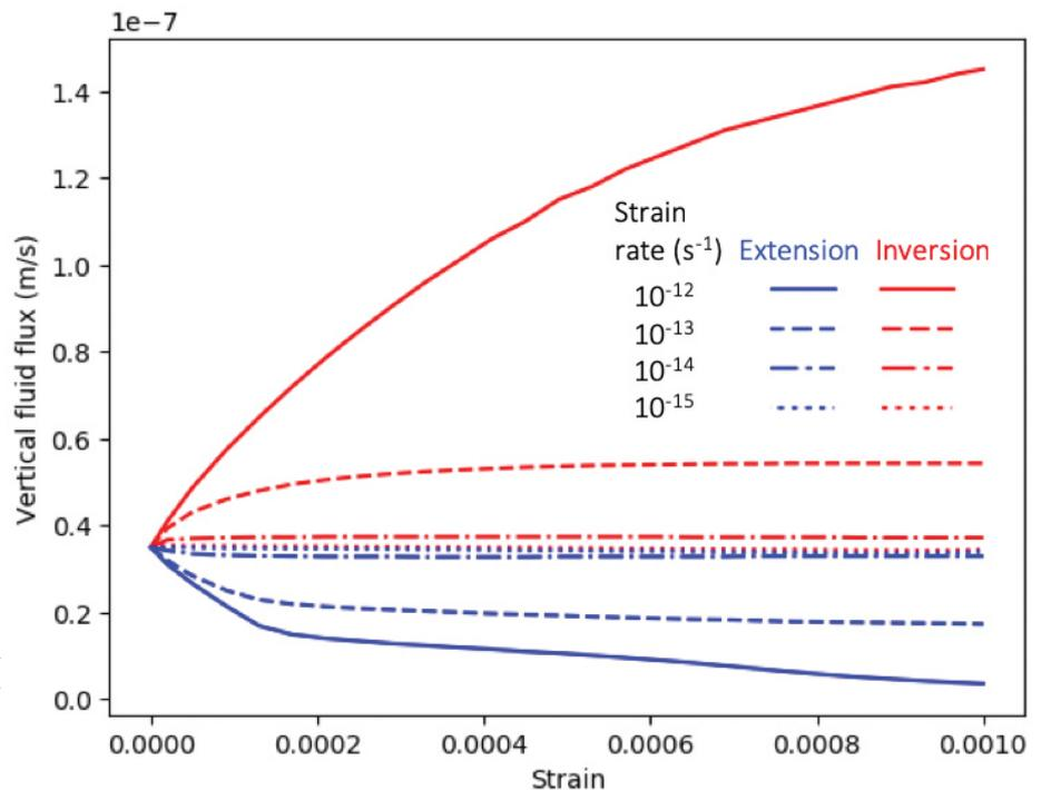
**Figure 4.** Effect of deformation on convection: Maximum vertical fluid flux in the faults as a function of strain rate.
