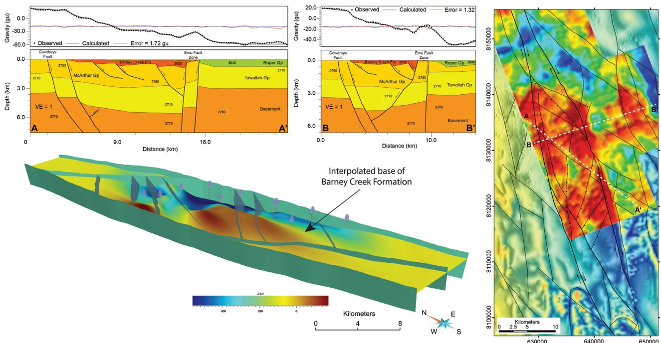
**Figure 4.** Architecture of the Glyde sub-basin determined from geophysical interpretation and modelling. (a–b) Forward modelled cross-sections of the Glyde sub-basin. c) Falcon gravity data (acquired by Armour Energy 2013) overlain with interpreted faults. (d) 3D model of the Glyde sub-basin showing location of wells, major faults and an interpolated surface for the base of the Barney Creek Formation.
