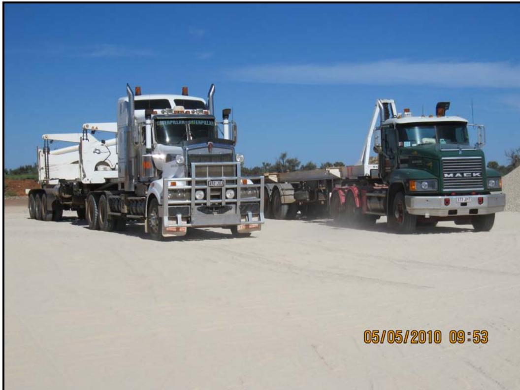
Photograph 7 – Side-lifter and Tipping Skel.
