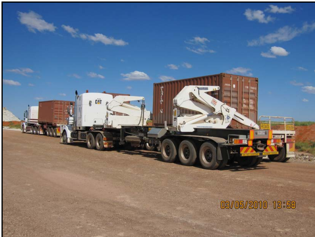
Photograph 8 – Lifting full containers from road train onto side-lifter.
