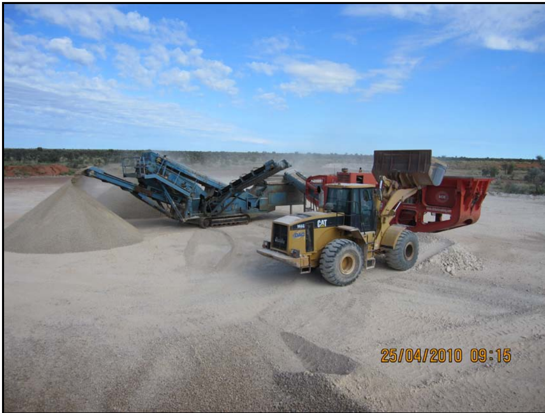
Photograph 5 - Re-crushing DSO "Intermediates" – combining crushing plant and screening plant.
