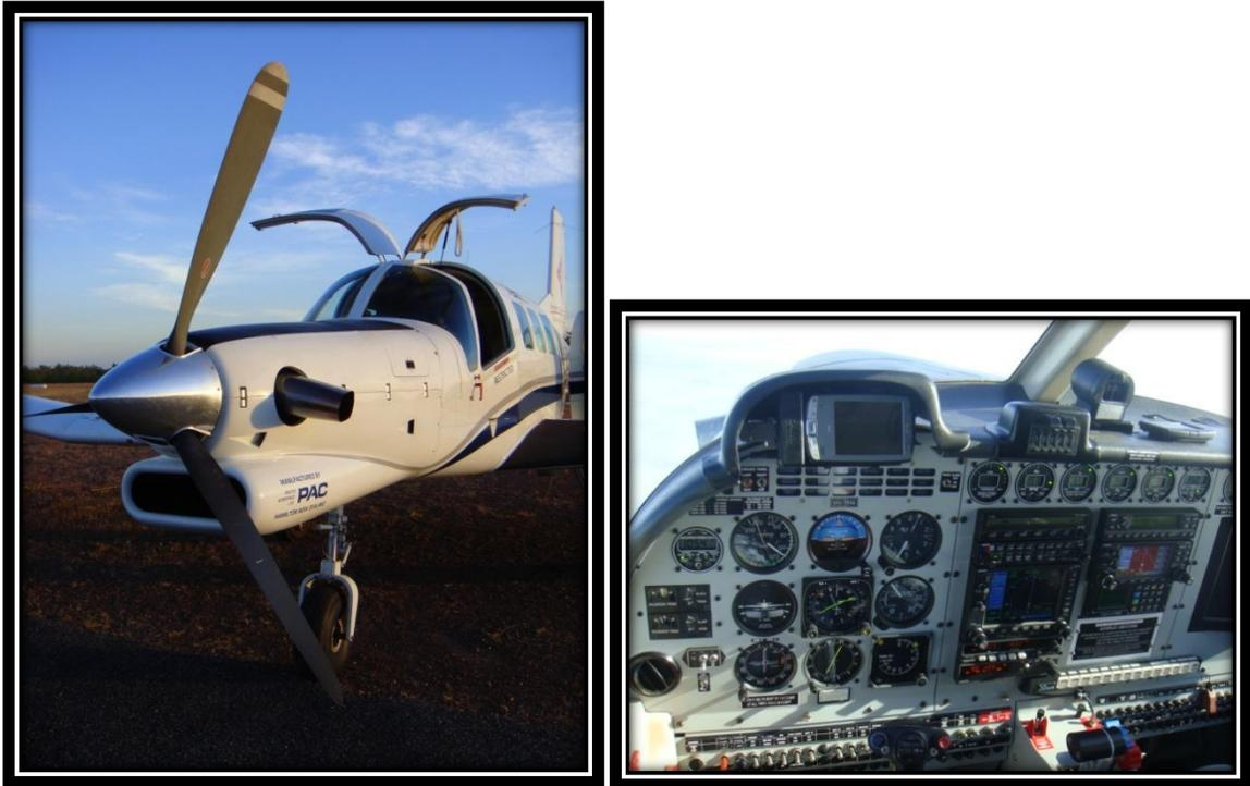
Our PAC750-XL, VH-TEQ was used as the survey platform. This aircraft combines good maneuverability with the benefits of a magnetically clean base for minimal interference with the magnetic performance of the sensor. The PAC750 is designed specifically to be flown at very low altitudes due to its agricultural background.
