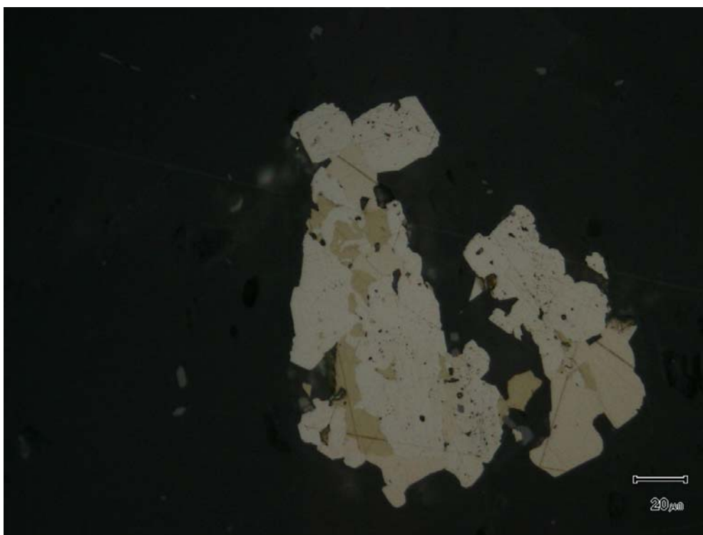
Fig 2 15546 PS (x50). Small composite sulphide grains with yellowish chalcopyrite and (in this photo) slightly pinkish possible pentlandite, all as inclusions in pale pyrite host.
