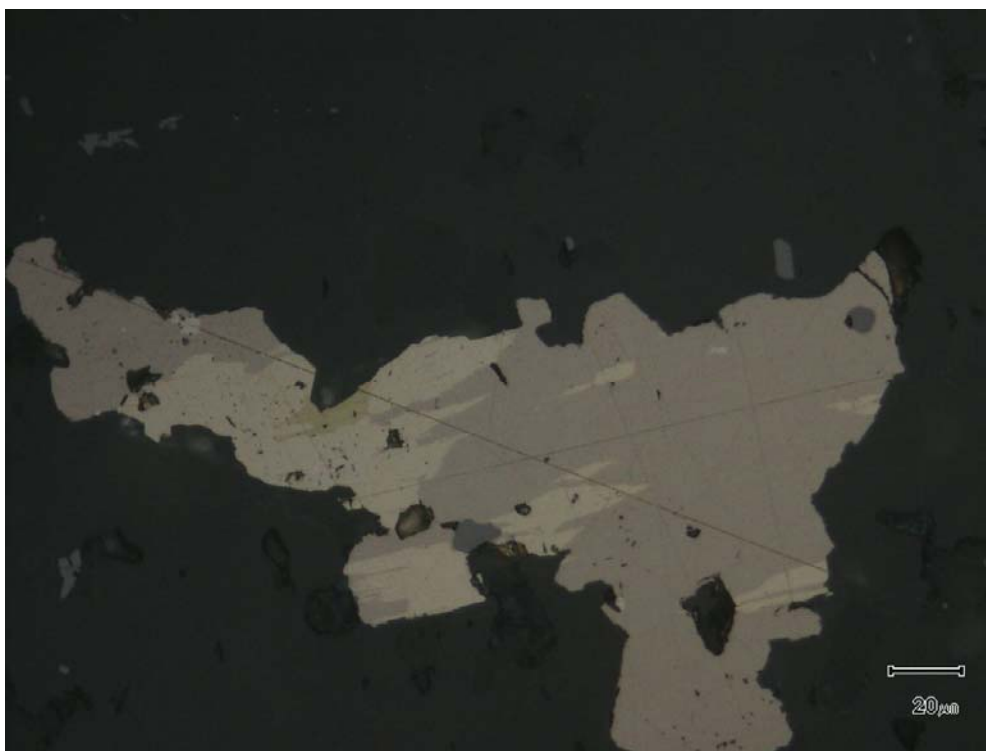
Fig 1 15546 Reflected light (RL)/polished section (PS). Magnification (x500). Composite sulphide grain of greyish-brown pyrrhotite incorporating cream coloured partly flame-like intergrowths of pentlandite, locally with sparse yellowish chalcopyrite.
