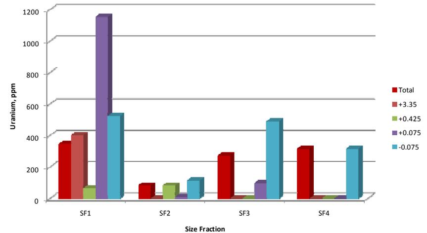
**Figure 3: Uranium distribution in post bottle roll test residues at different size fraction**
