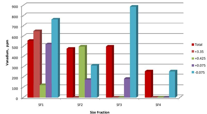
**Figure 4: Vanadium distribution in post bottle roll test residues at different size fraction**
