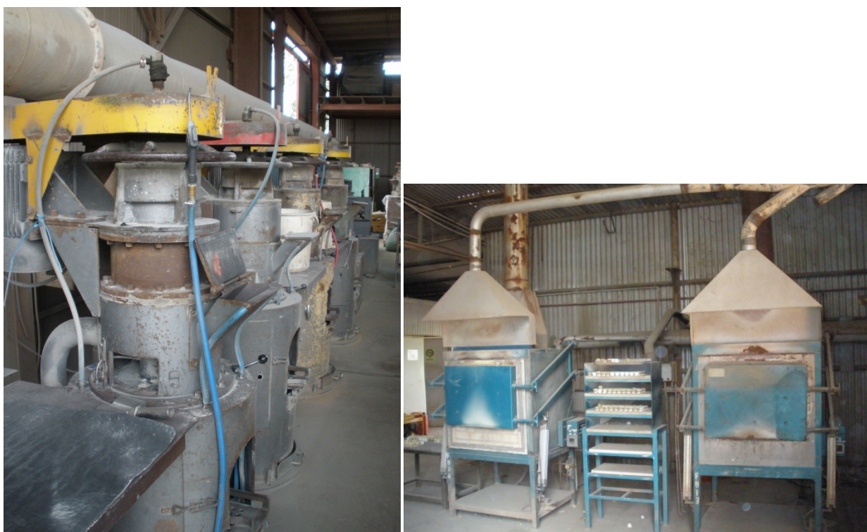
Figure 4-7 Keegor grinding mills and fusion furnaces
