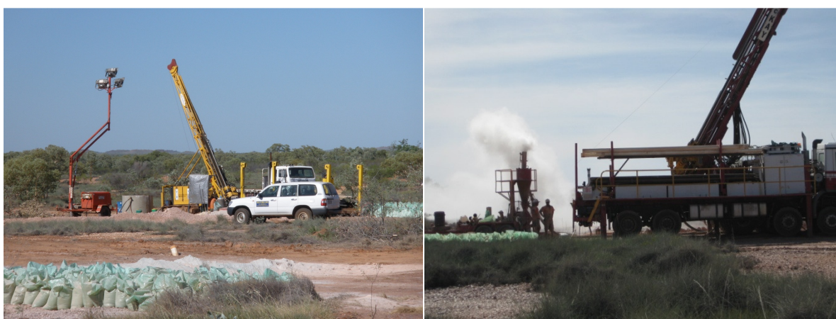
Figure 4-2 Diamond core and RC drilling in progress at Juno.
