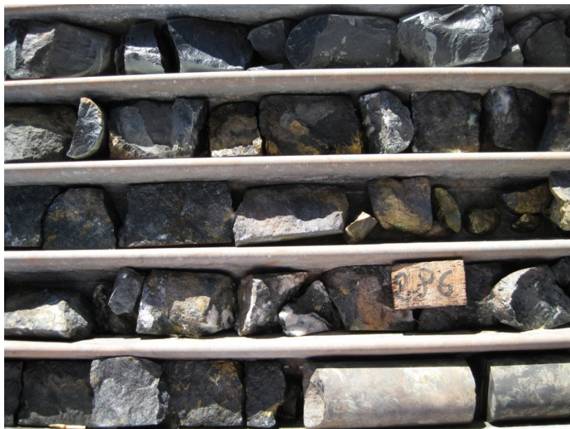
Figure 4-4 Historical underground core from hole JD900078, ironstone with minor quartz veinlets and chalcopyrite (286 feet down-hole).
