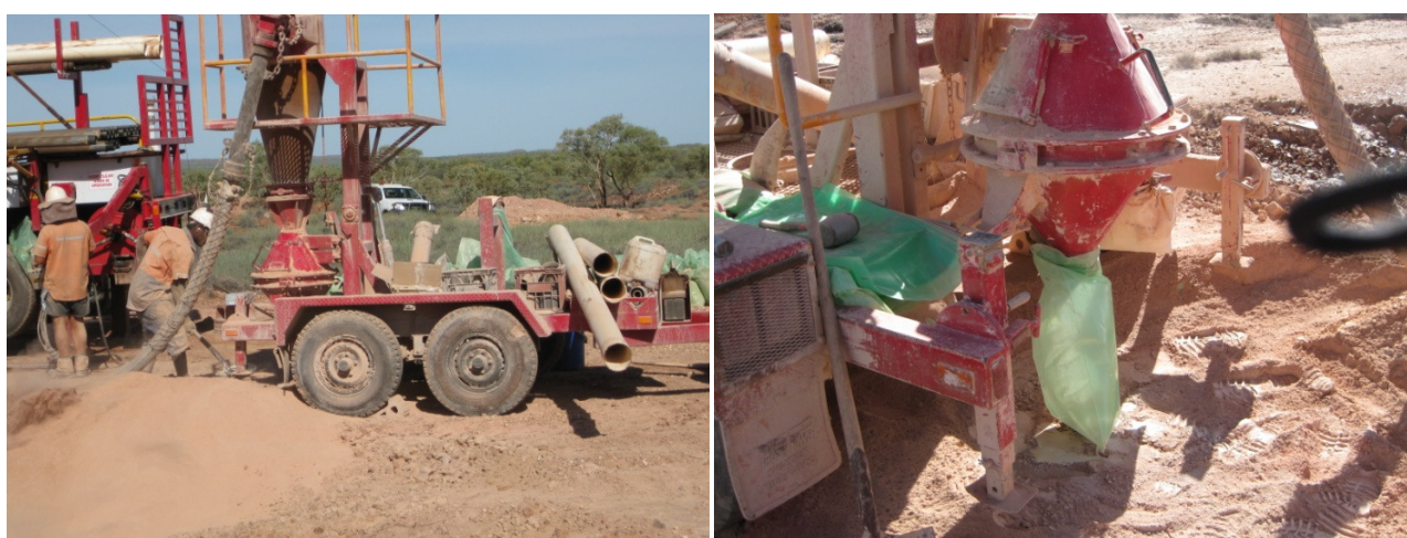
Figure 4-3 Collection of RC bulk sample from the trailer mounted cone splitter.
