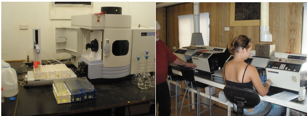
Figure 4-8 ICP-OES Spectrometer and Fire Assay AAS.
