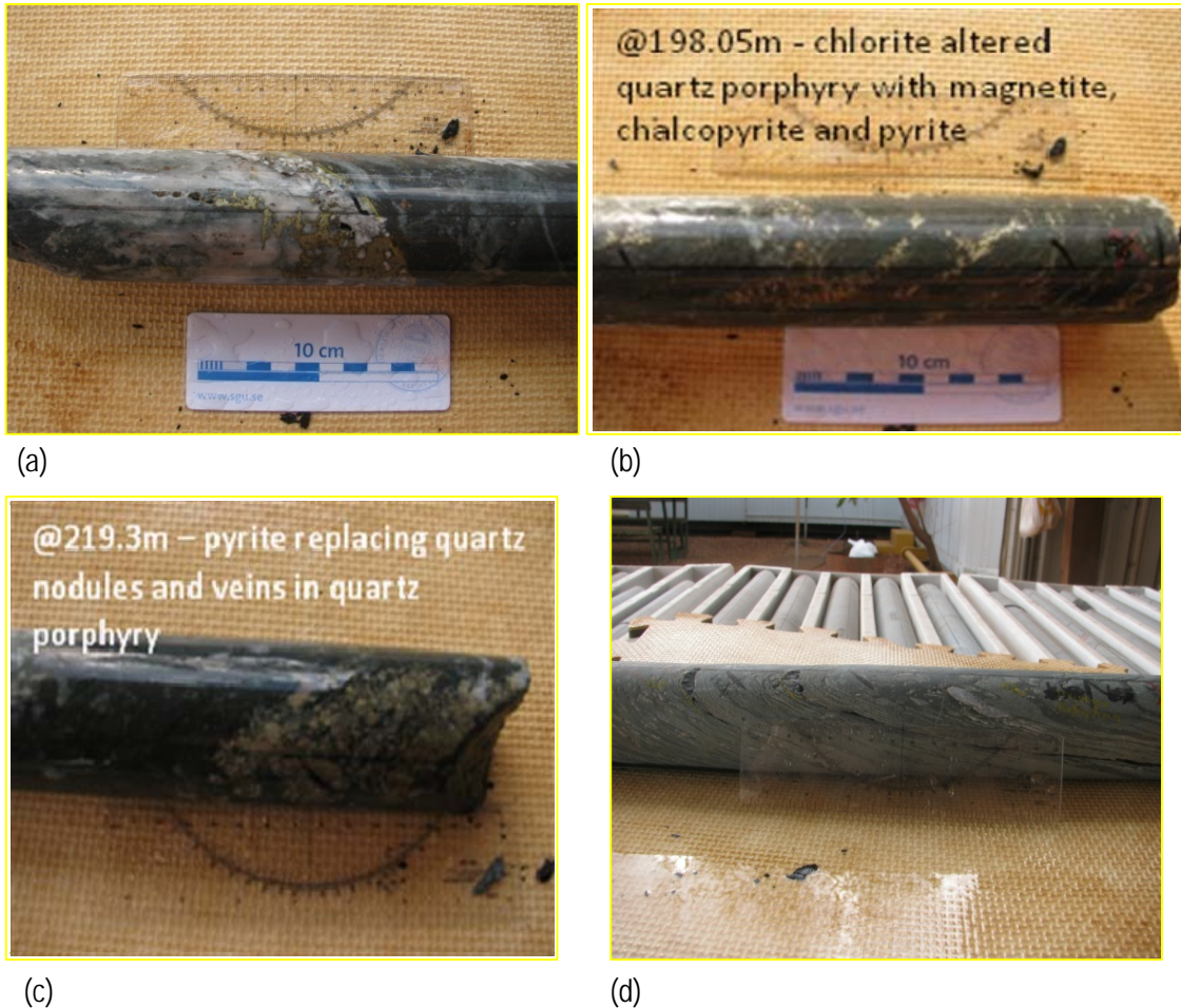
Core photos of CBDD003. (a) 192.85m – quartz vein with chalcopyrite and pyrite in contact with magnetite; (b) 198.05m - chlorite altered quartz porphyry with magnetite, chalcopyrite and pyrite; (c) 219.3m – pyrite replacing quartz nodules and veins in quartz porphyry; (d) 221.7m – strongly foliated quartz porphyry.
