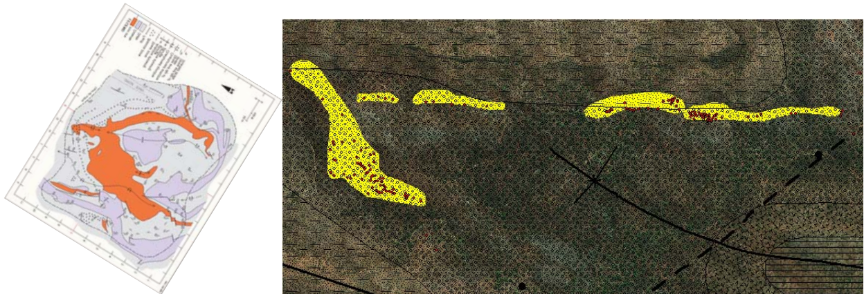
Figure 10 – Geological map (Ferenczi, P.A., 2001) of Helene 6/7 flipped, rotated and equal scaled for comparison (left). Outcropping mapped hematite beds and sample locations (right).
