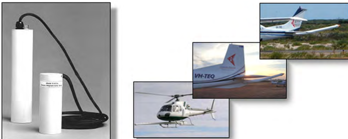
Figure 6 G822A Magnetometer and Typical Stinger Mounts
