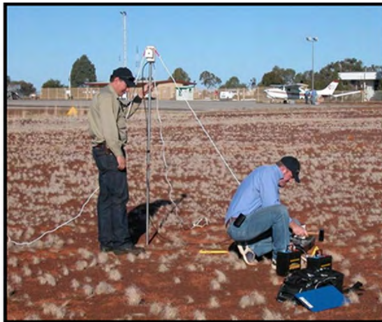
Figure 12 Setting up base station magnetometer
