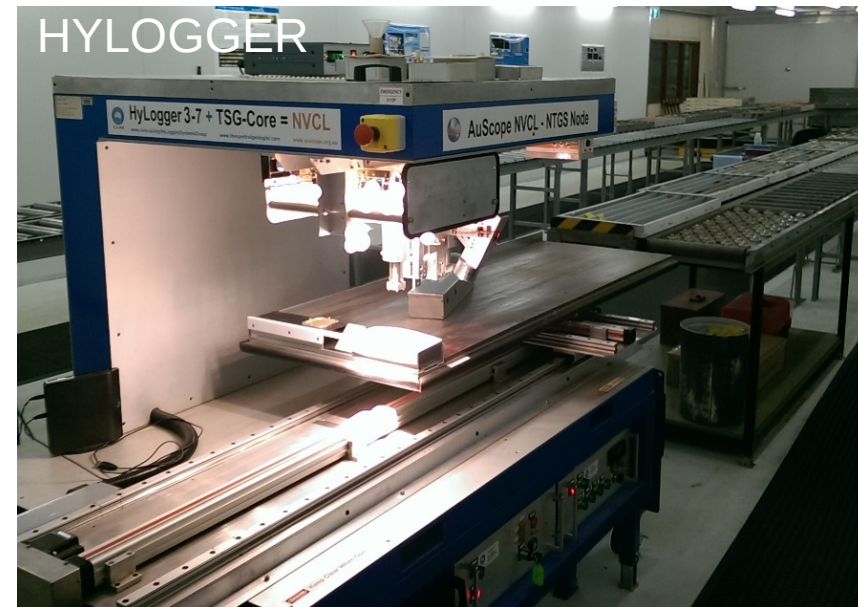
Proximal automatic / continuous drillcore / rock samples; Hyperspectral (mineral species including quartz, feldspars, pyroxenes) with imagery (HyLogger)
