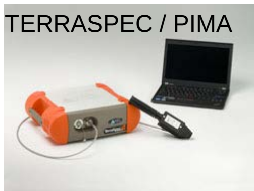
Proximal manual / point measurement (no imagery, less minerals detected than HyLogger)
