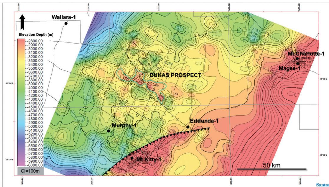
Figure 7. Current depth converted basement map showing Dukas Prospect depth closure polygon.
