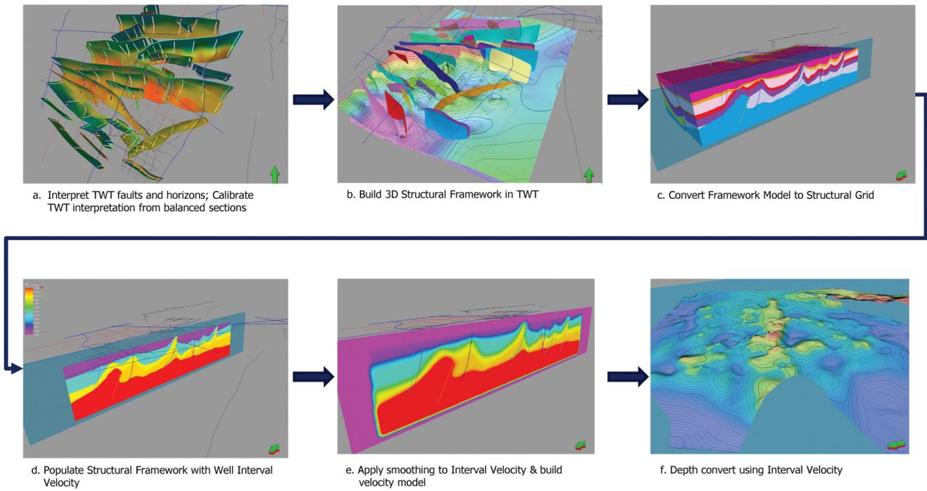
Figure 4. Building the 3D framework model and time to depth conversion workflow.
