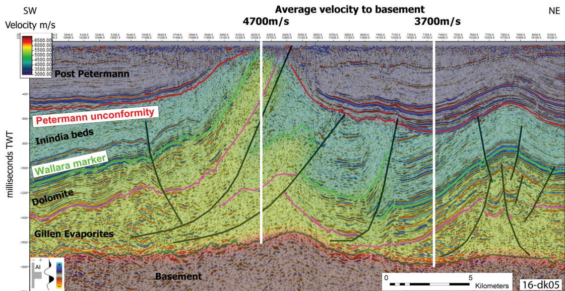
Figure 6. Seismic profile AMSAN 16-DK05 with modeled velocity showing as much as 20% variation in average velocity to basement. Seismic line location in Figure 1.
