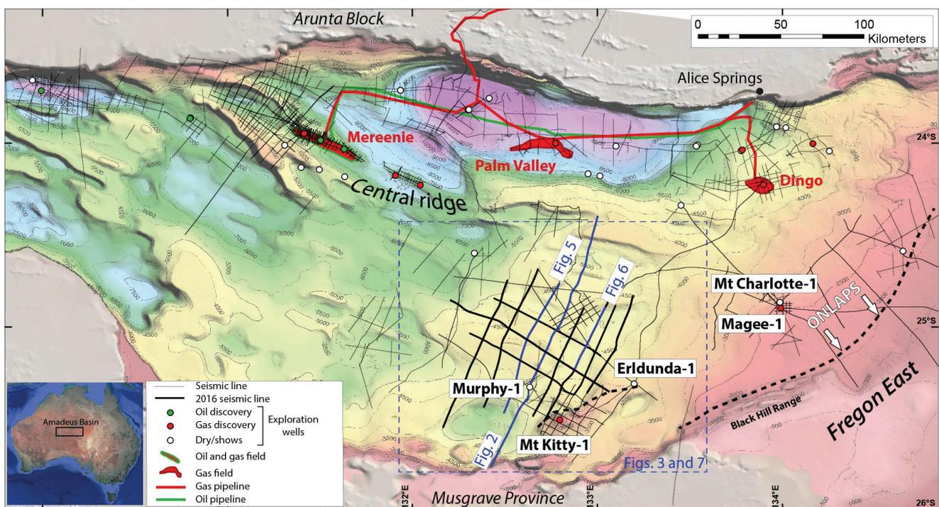
**Figure 1.** Overburden map (in metres) of the Amadeus Basin derived from SEEBASE® depth-to-basement model (FROGTECH 2015, Debacker *et al* 2016) showing seismic and wells.
