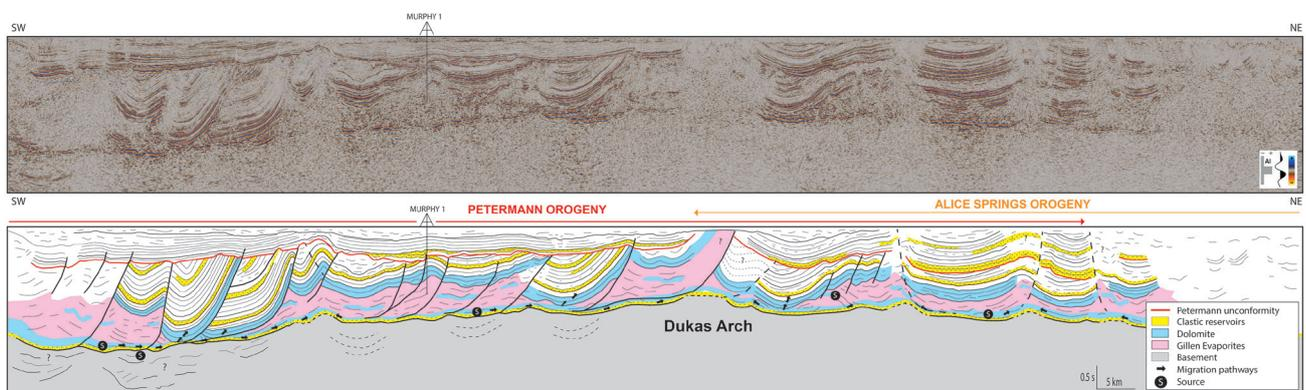
**Figure 2.** Seismic line AMSAN13-B04 and associated line drawing across the southern Amadeus Basin showing structural detachment in the Gillen Formation evaporites. Seismic line location in Figure 1.
