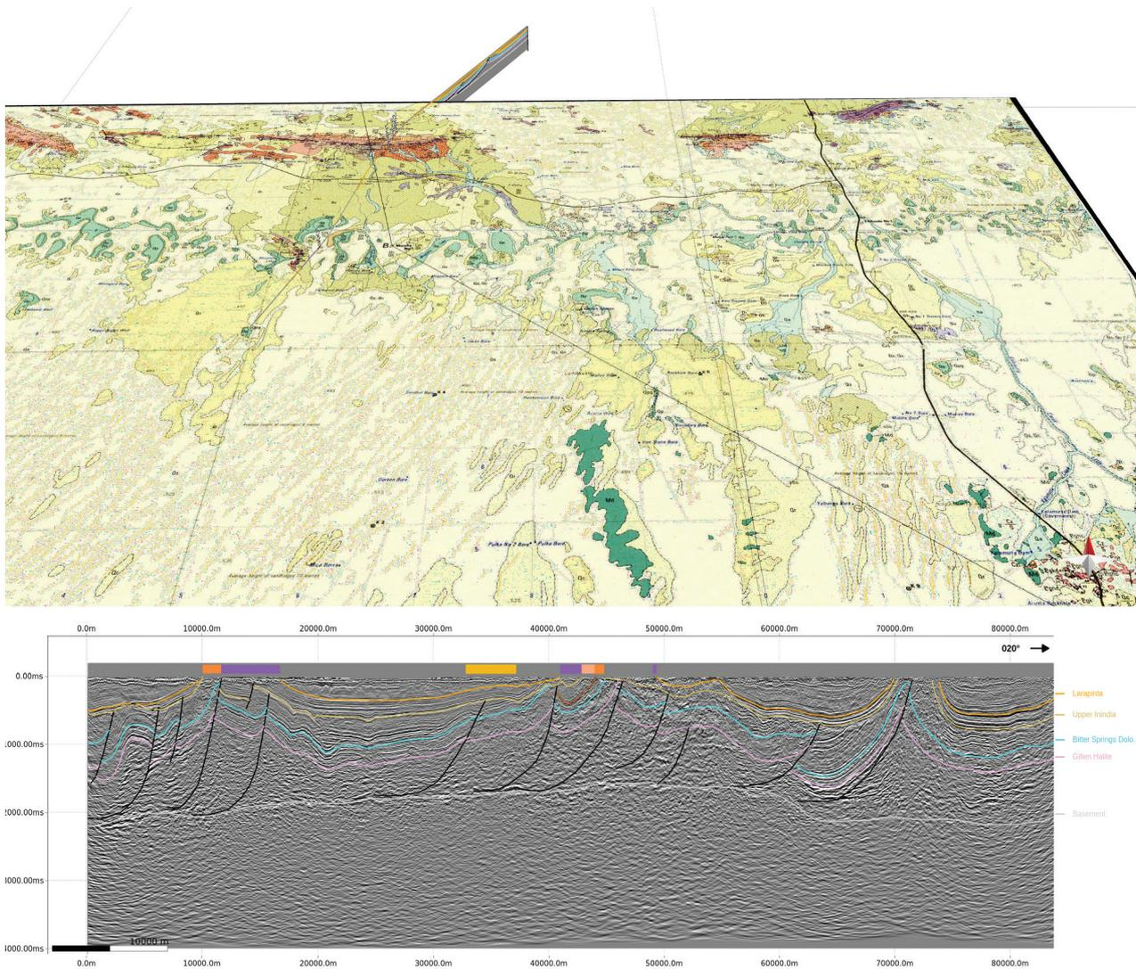
Figure 5. Integration of surface geology into 2D seismic interpretation – AMSAN16-DK03 example.
