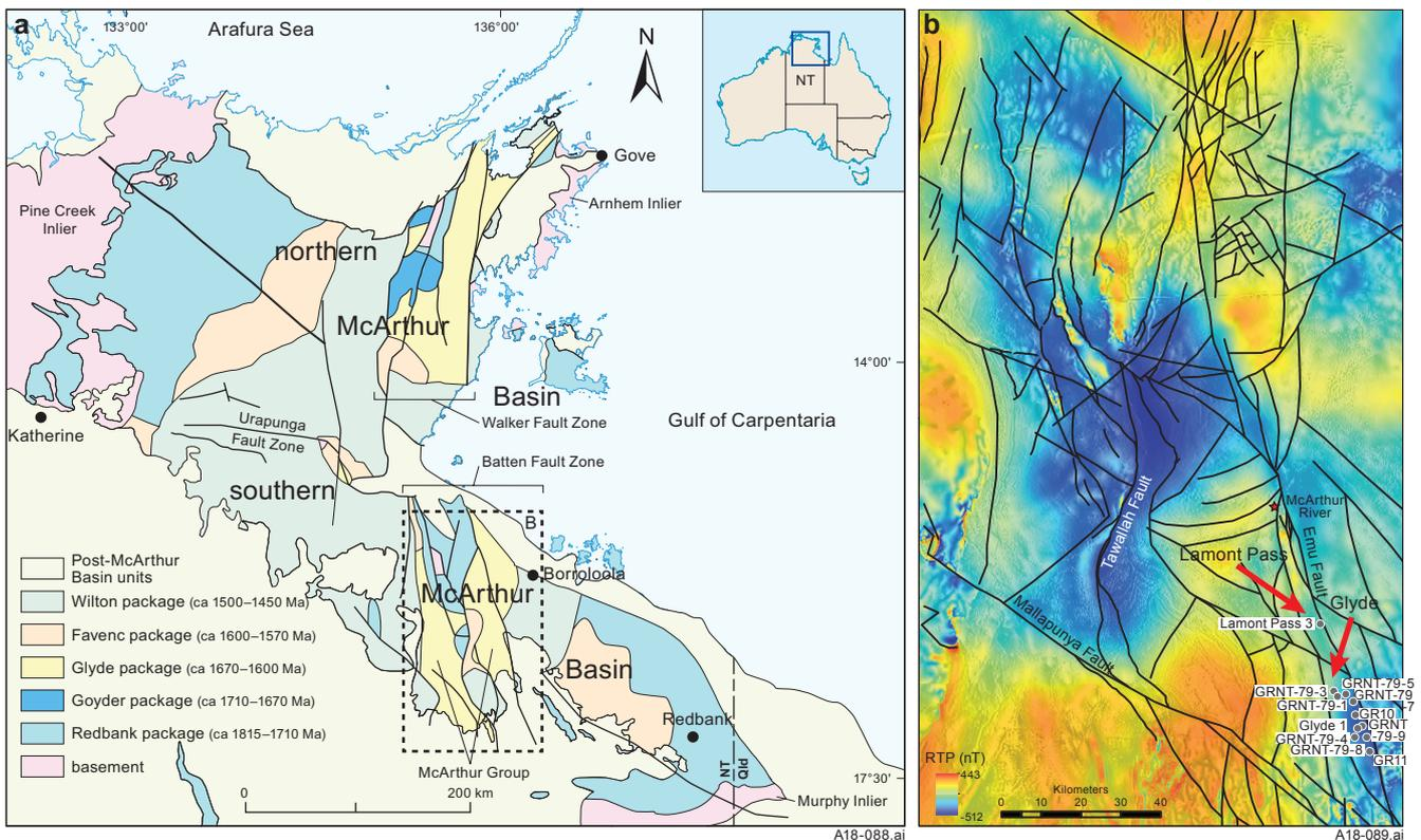
**Figure 1.** Simplified geological map of the McArthur Basin and magnetics of the Batten Fault Zone. (a) Spatial distribution of depositional packages across the McArthur Basin (modified after Ahmad *et al* 2013, Rawlings 1999). (b) Magnetics of the Batten Fault Zone showing the location of the Glyde sub-basin, Lamont Pass palaeohigh, and drillholes used in this study.
