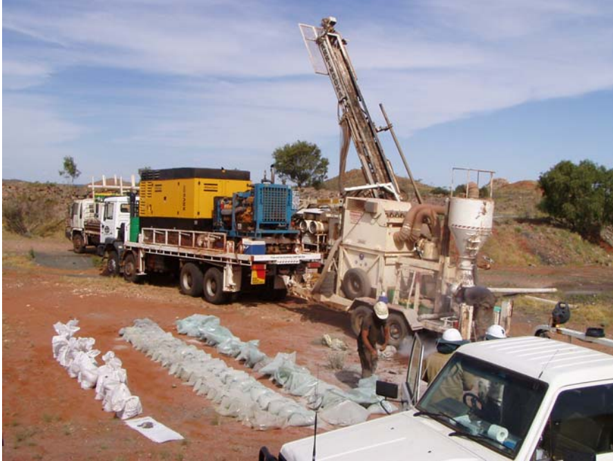
Figure 1: Drilling rig, with cyclone and splitter hitched behind the booster truck
