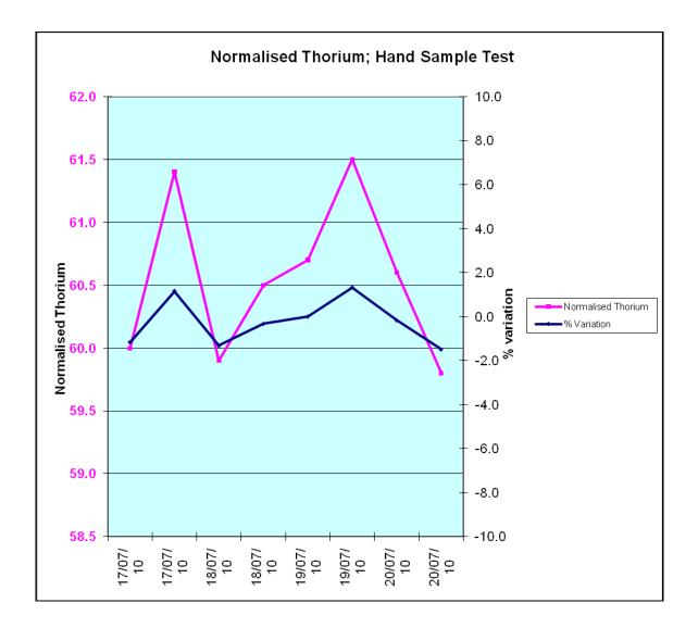
b) A Test Line was flown at the same height as the survey specified height to verify magnetometer, spectrometer and barometric altimeter baselines. The test line was flown over a repeatable line of five kilometers and was flown in either direction. The test line Thorium window counts fell within a 10% envelope (+/- 5% of the mean over the survey period).
