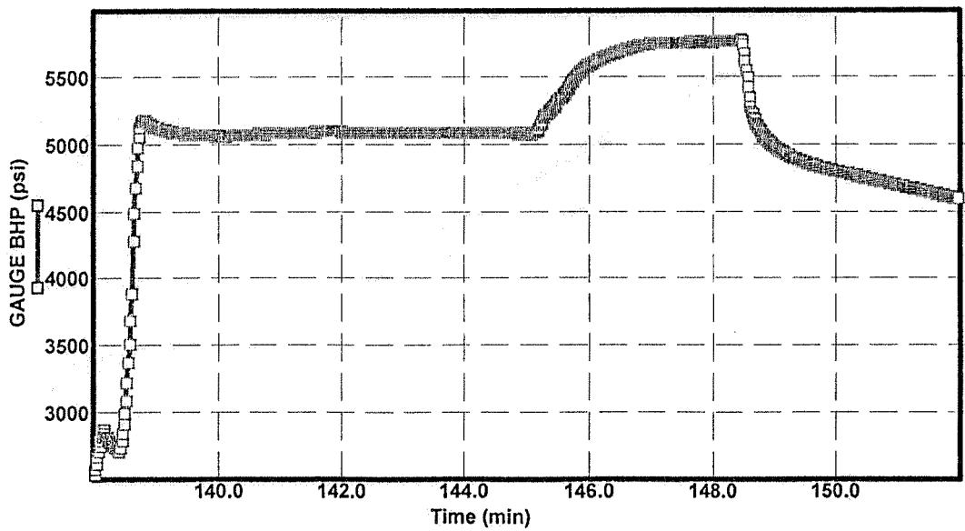
**FIG. 14 - Boragel minifrac/SI BHP record,
