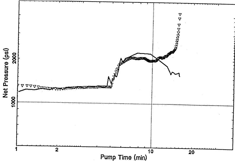
**FIG. 29 - Treatment net BHTP history match with design model, E. Mereenie #41 (P4).**
