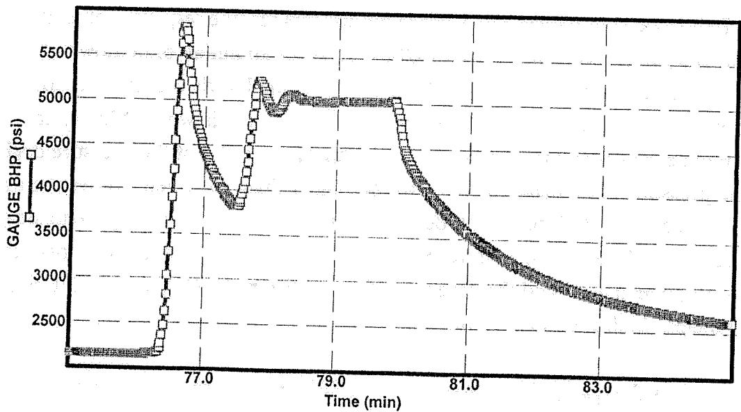
**FIG. 3 - Slick water PI/SI test BHP record,
