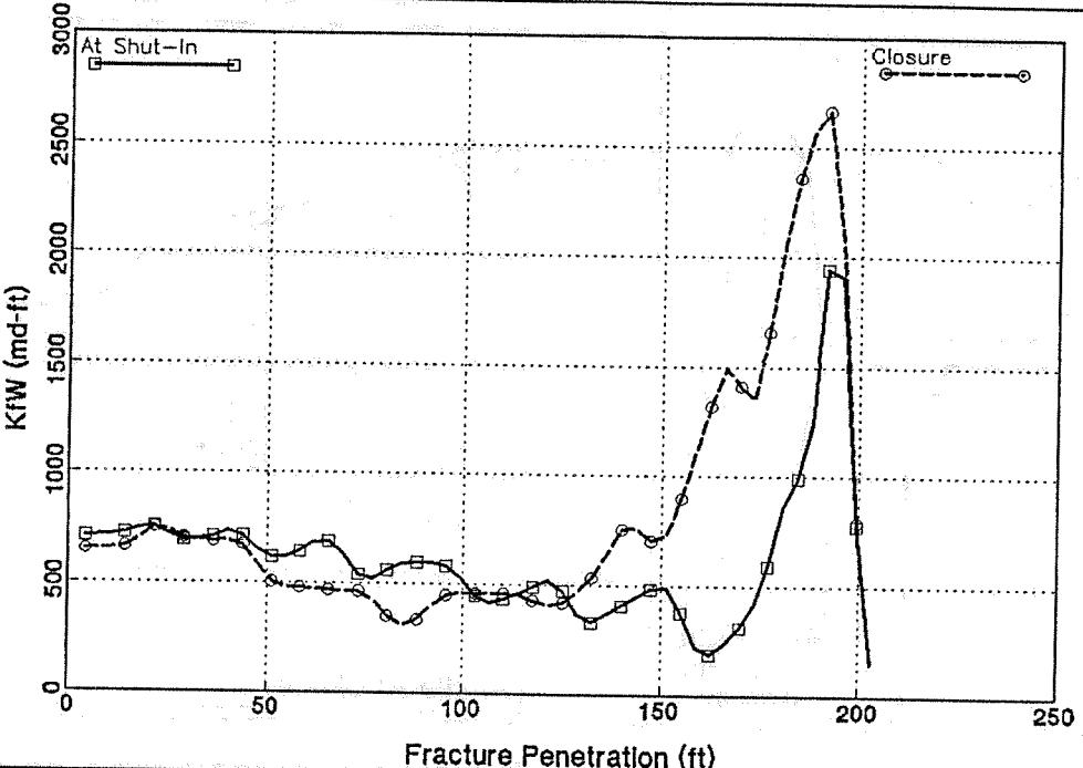
**FIG. 25 - Final treatment design predicted in-situ conc., E. Mereenie #41 (P4).**
