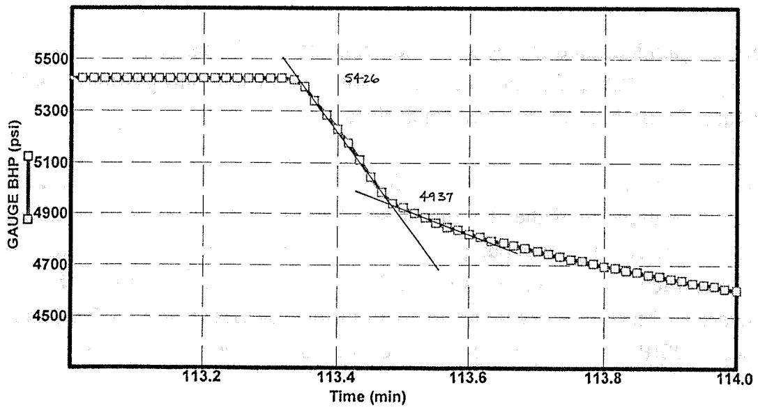
**FIG. 9 - Slick water SRT/SI BH ISIP evaluation,
