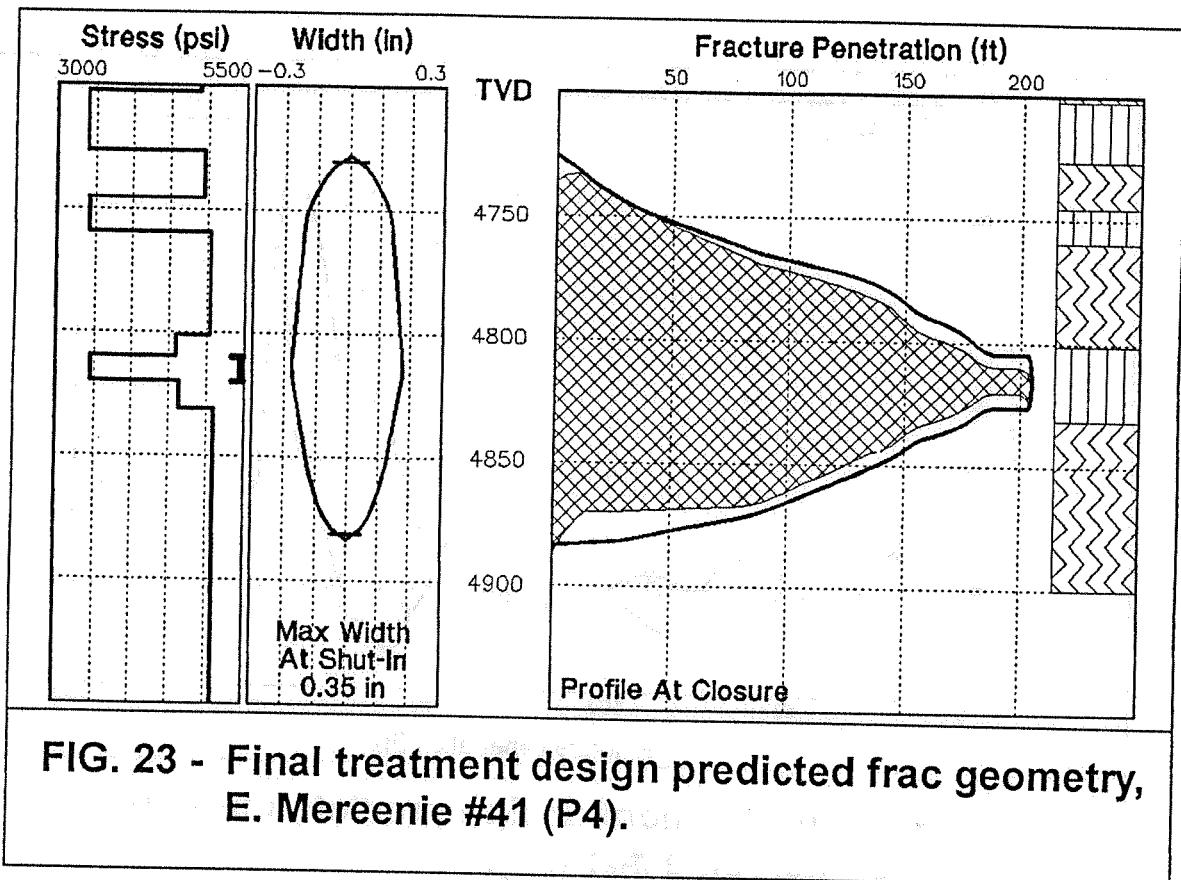
**FIG. 23 - Final treatment design predicted frac geometry,
