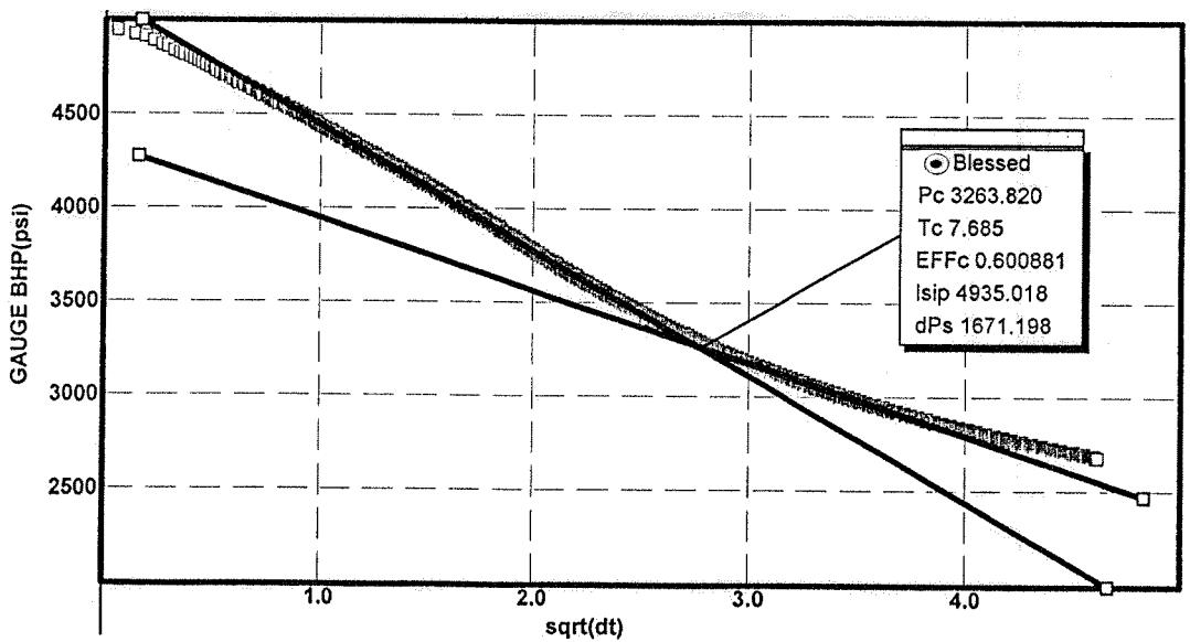
**FIG. 12 - Slick water SRT/SI BH sq.rt. SI time plot #2,
