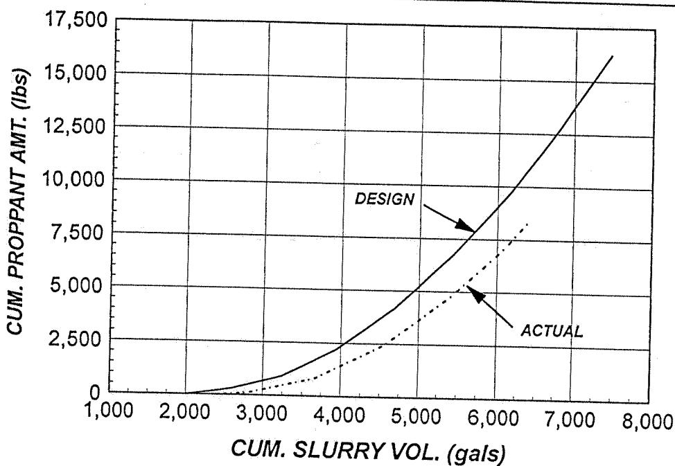
**FIG. 27 - Comparison of actual to design prop schedule, E. Mereenie #41 (P4).**
