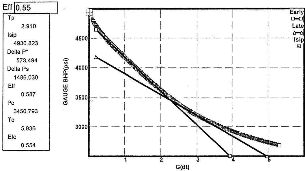
**FIG. 13 - Slick water SRT/SI BH G-function plot,
