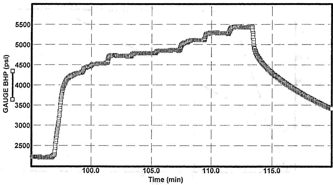
**FIG. 8 - Slick water SRT/SI BHP record,
