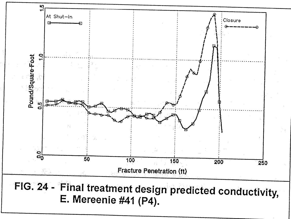
**FIG. 24 - Final treatment design predicted conductivity,
