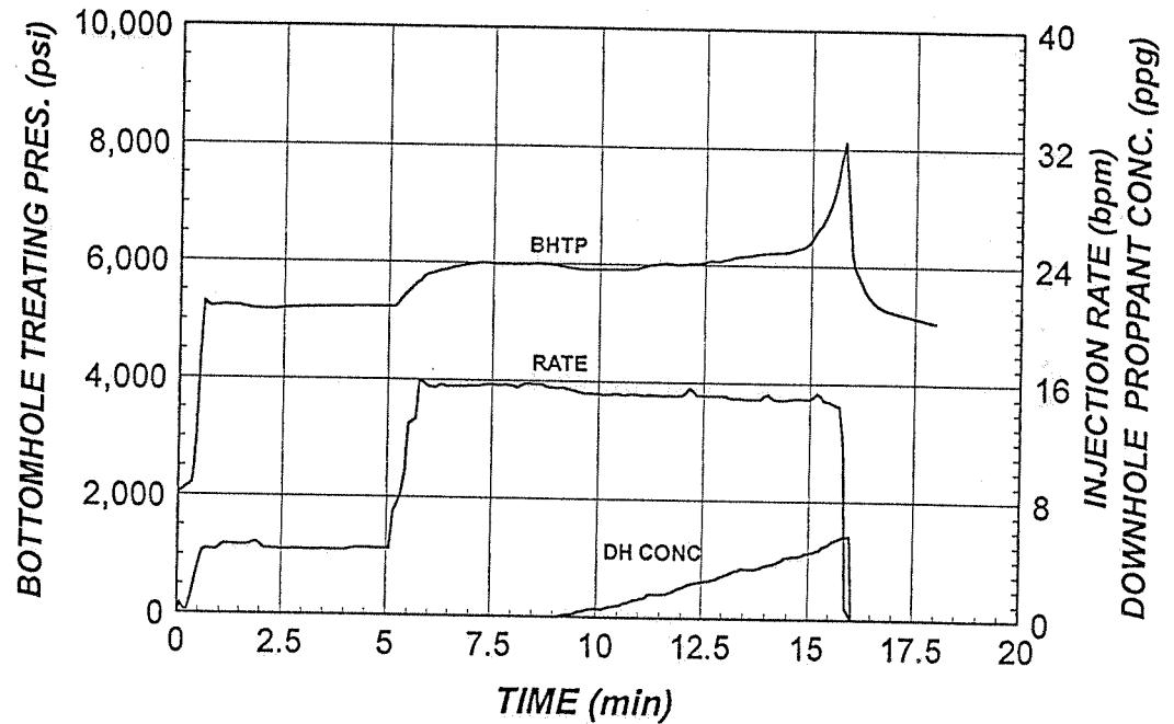
**FIG. 28 - Treatment summary of bottomhole parameters, E. Mereenie #41 (P4).**
