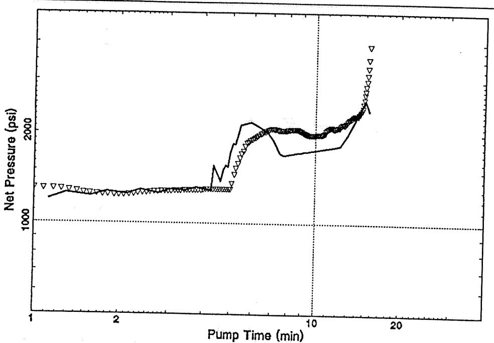
**FIG. 33 - Treatment net BHTP history match w/ increased P4 leak-off, E. Mereenie #41 (P4).**
