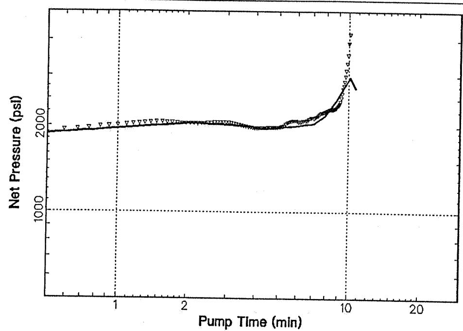
**FIG. 34 - Treatment net BHTP history match of crosslinked gel portion only, E. Mereenie #41 (P4).**
