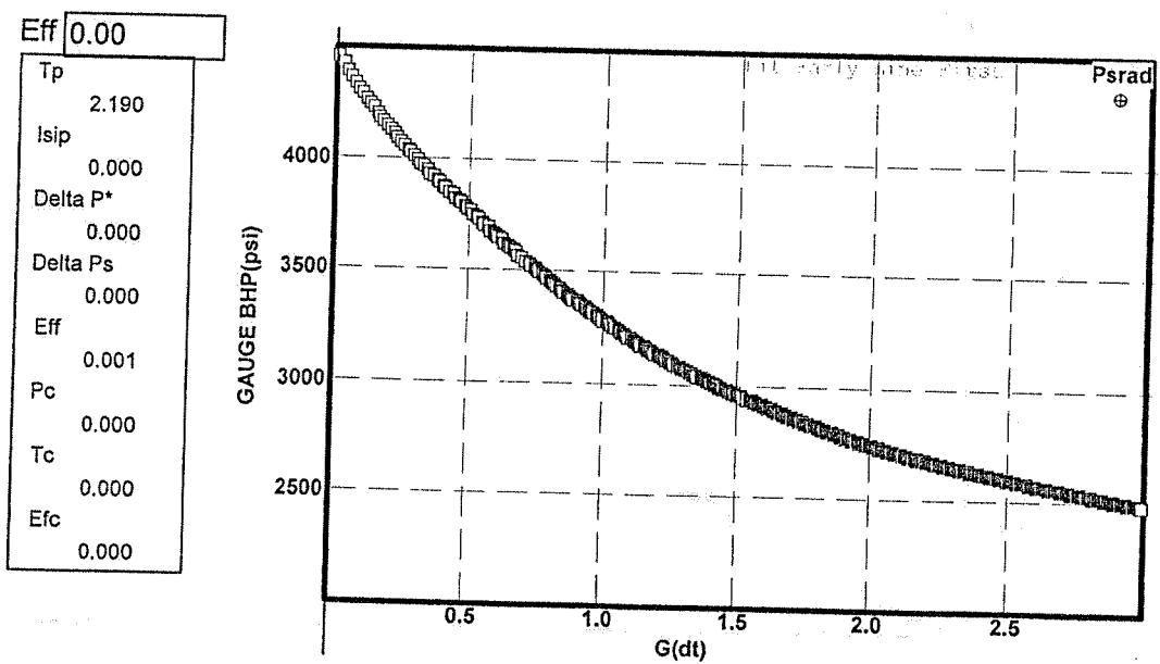
**FIG. 7 - Slick water PI/SI test BH G-function plot,
