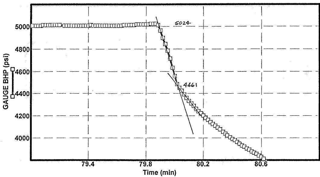
**FIG. 4 - Slick water PI/SI test BH ISIP evaluation,
