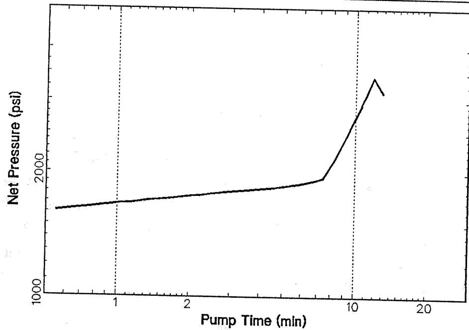
**FIG. 22 - Final treatment design predicted net BHTP,
