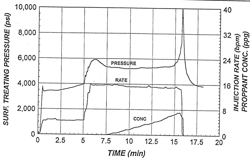
**FIG. 26 - Treatment summary of surface parameters, E. Mereenie #41 (P4).**
