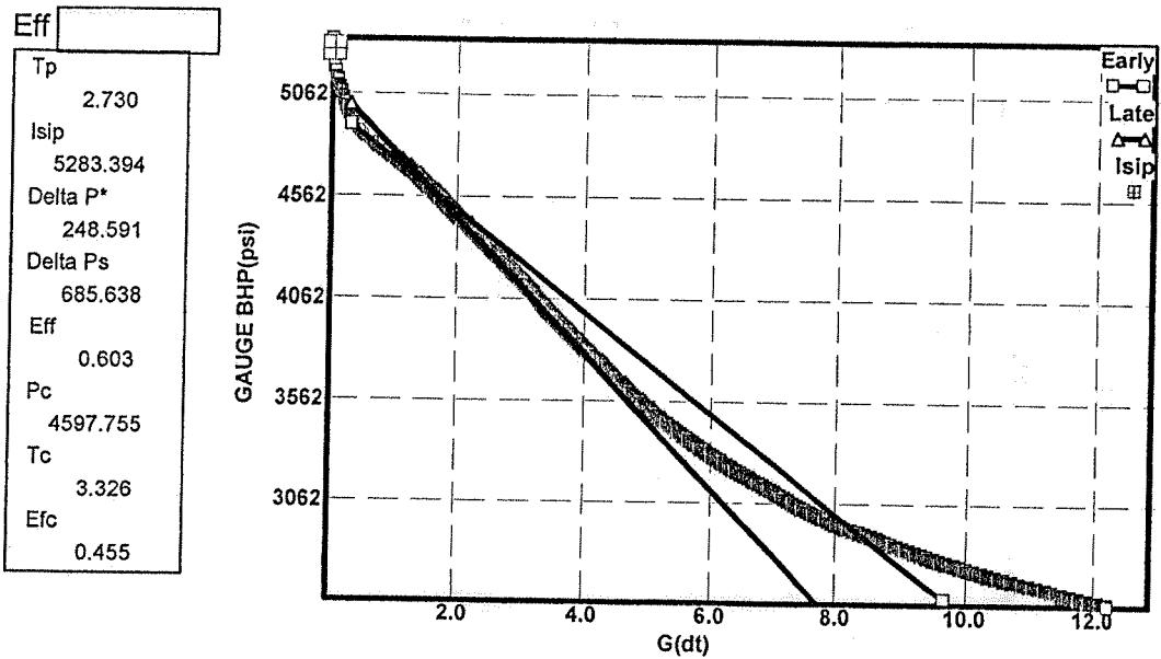
**FIG. 17 - Boragel minifrac/SI BH G-function plot #1,
