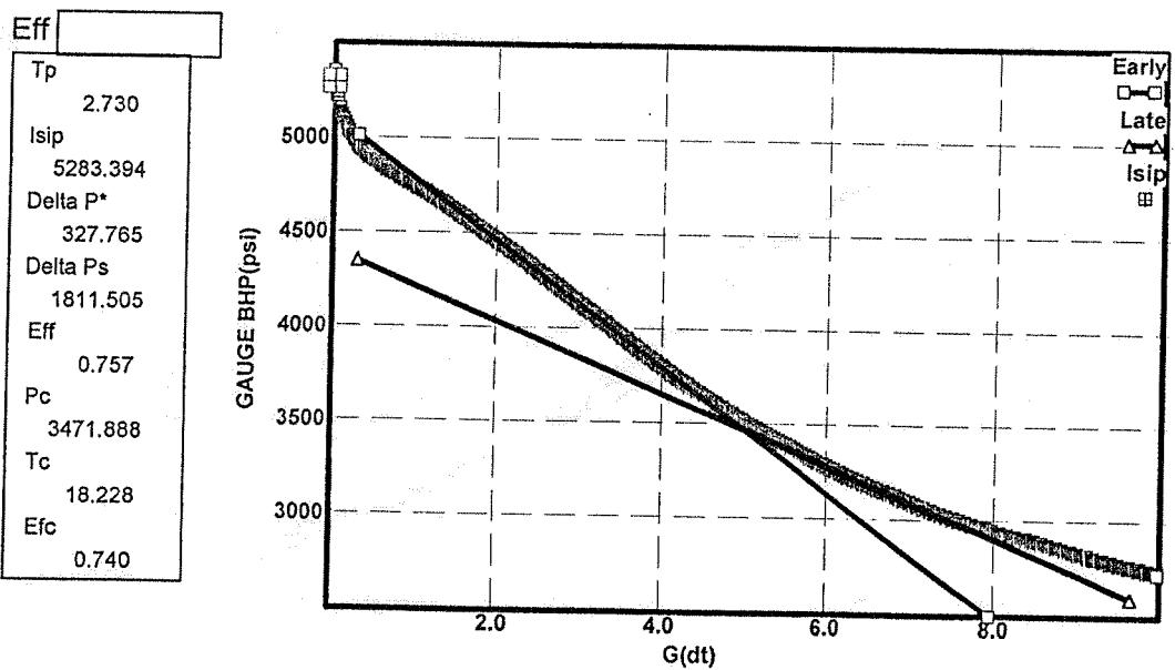
**FIG. 18 - Boragel minifrac/SI BH G-function plot #2,
