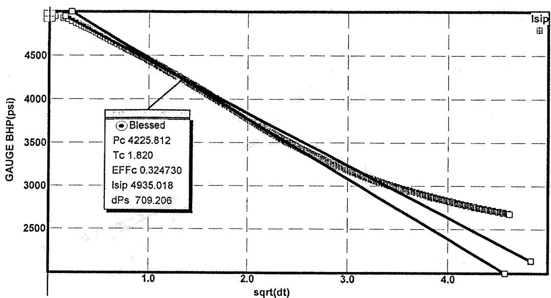
**FIG. 11 - Slick water SRT/SI BH sq.rt. SI time plot #1,
