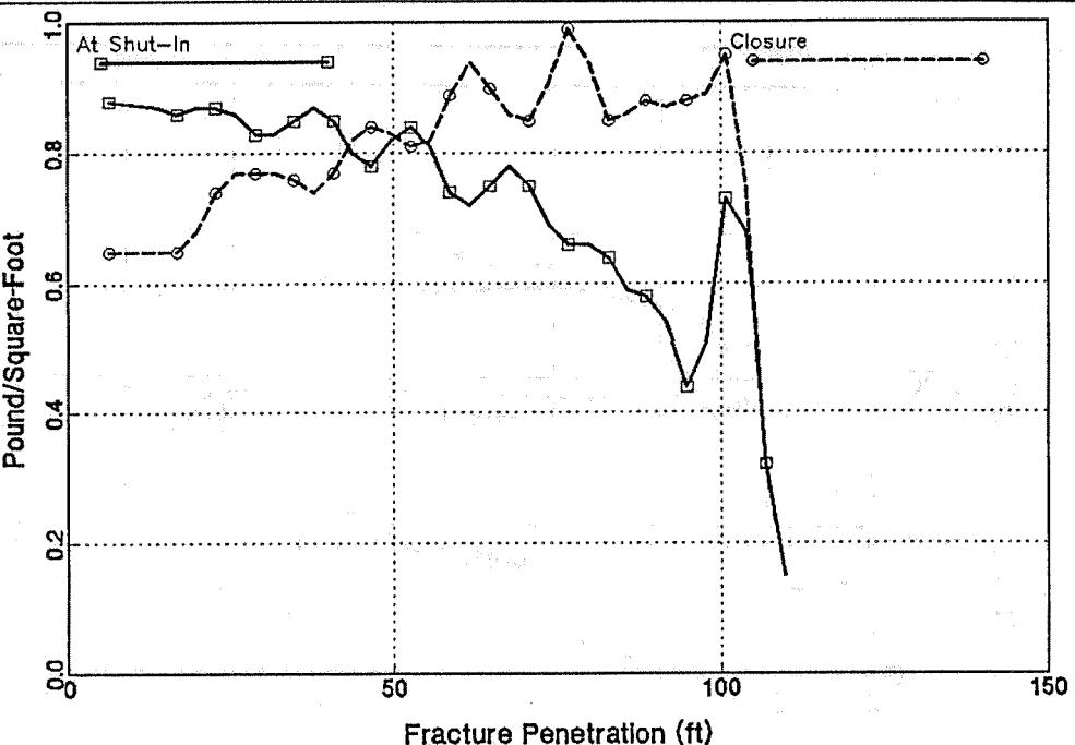
**FIG. 23 - Final treatment design predicted in-situ conc., E. Mereenie #41 (P3-190/230/250).**
