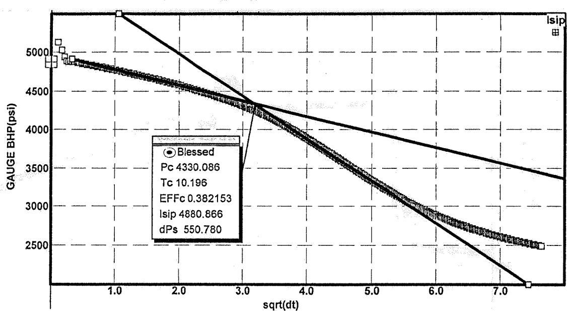
**FIG. 11 - Slick water SRT/SI test BH sq.rt. SI time plot,
