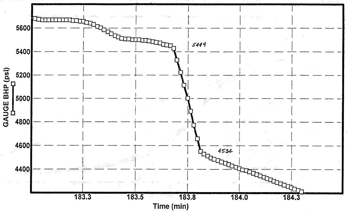
**FIG. 4 - Slick water PI/SI test BH ISIP evaluation,
