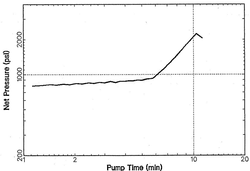
**FIG. 20 - Final treatment design predicted net BHTP,
