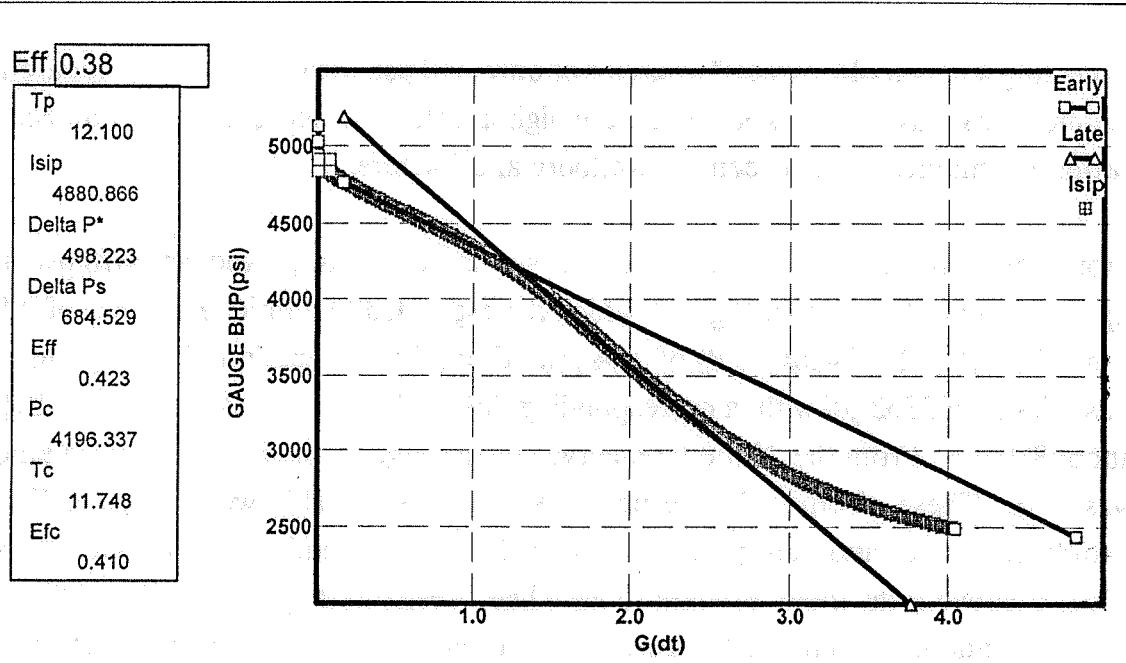
**FIG. 12 - Slick water SRT/SI test BH G-function plot,
