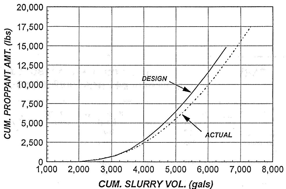
**FIG. 25 - Comparison of actual to design prop schedule, E. Mereenie #41 (P3-190/230/250).**
