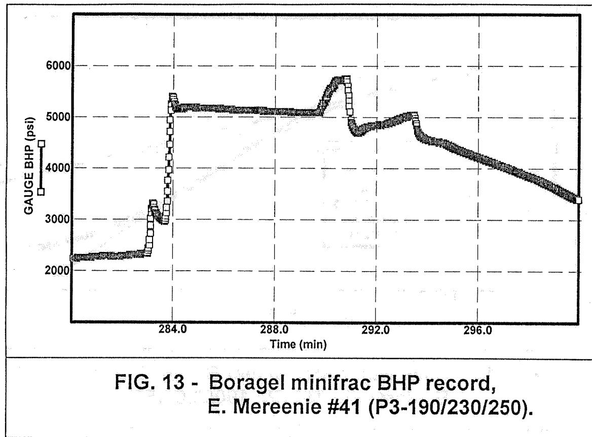
indicating a downhole "excess" pressure of only 318 psi. From this it was apparent that the more viscous crosslinked gel at the higher rate was successful in establishing far better communication between the wellbore and fracture.
