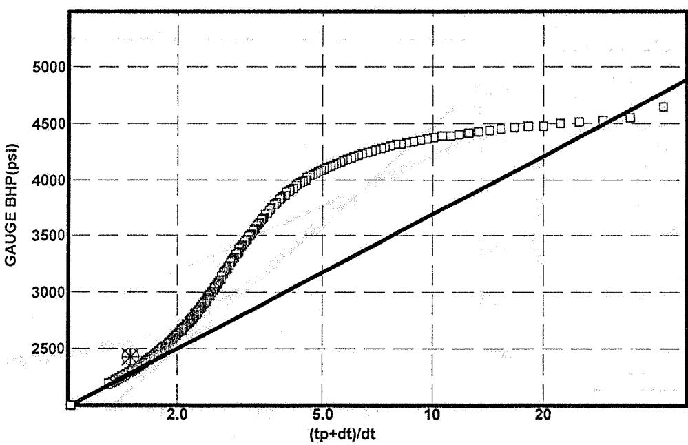
**FIG. 5 - Slick water PI/SI test BH Horner plot,
