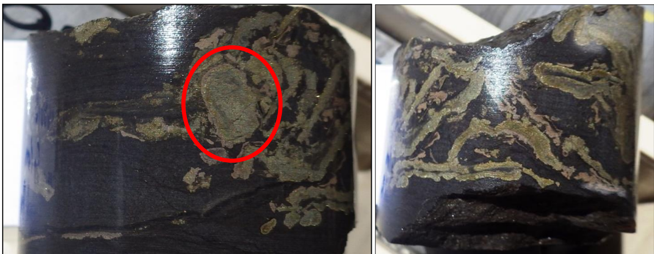
Figure 9. NB16DD018 @ 195.7 m: Left: light reddish brown sphalerite occurs as a rim surrounding a large pyrite aggregate; Right: sphalerite occurs as contorted bands parallel to hydrothermal pyrite bands; (NQ core 5 cm diameter).
