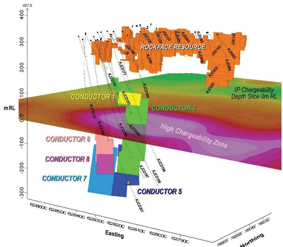
Figure 2. Rockface Prospect DHEM conductors and IP chargeability perspective view (looking southeast).
