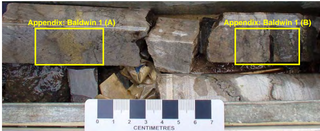
Figure 2: Copper-lead-zinc mineralisation in dolomitic limestone in Arthur Creek Formation (Baldwin 1; approximately 889.3 to 889.5m).
