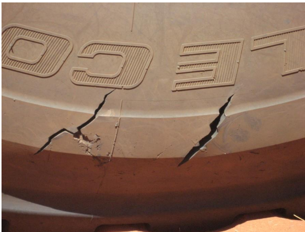
Photo 8: Result of dropping vib tyre pressure far enough to get over dunes
