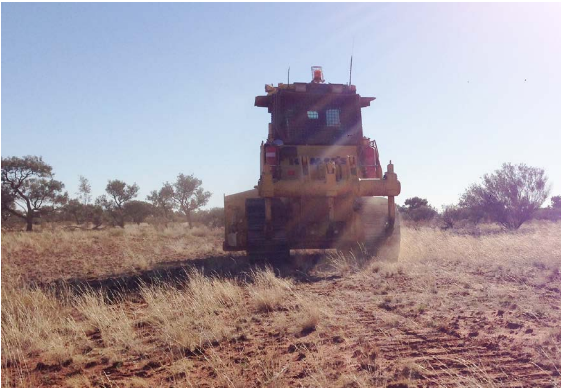
Photograph 3: Blade Up Technique for the line preparation
