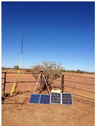
GPS Base Station, Radio antenna and Solar cells supplementing the battery power.
