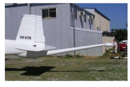
magnetometer were located within the tail stinger.
