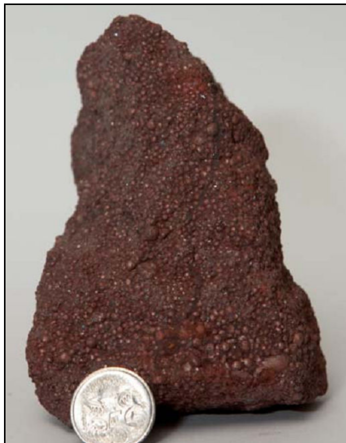
Plate 2: Cemented oolitic ore sample from the Roper Bar area (A. Wygralak collection; From Ahmad et al., 2013).
