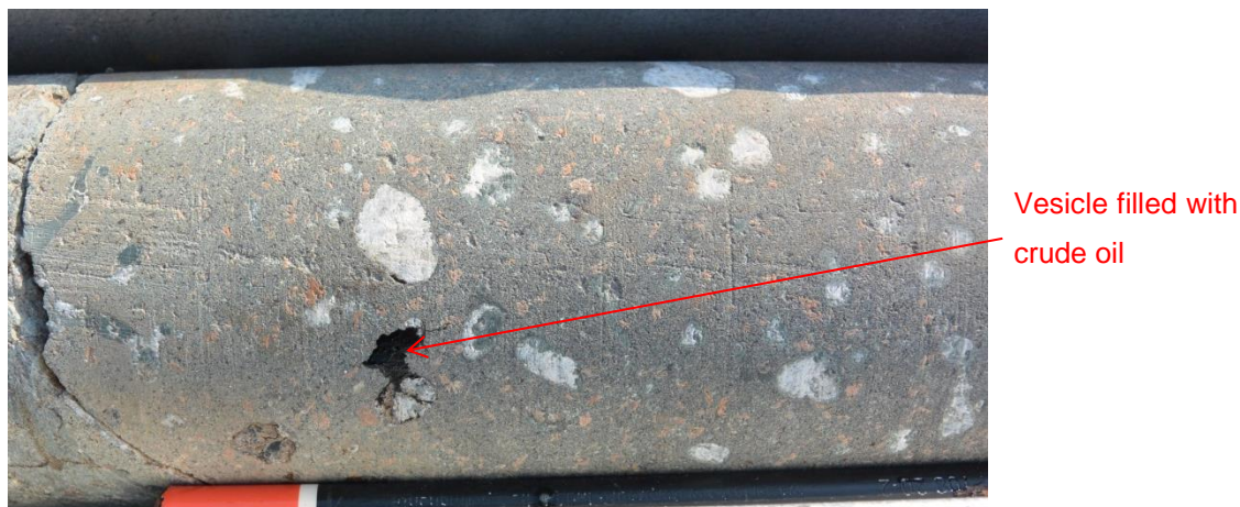
Figure 22: Photograph of vesicular basalt in SKDH05. Some vesicles were filled with crude oil.
