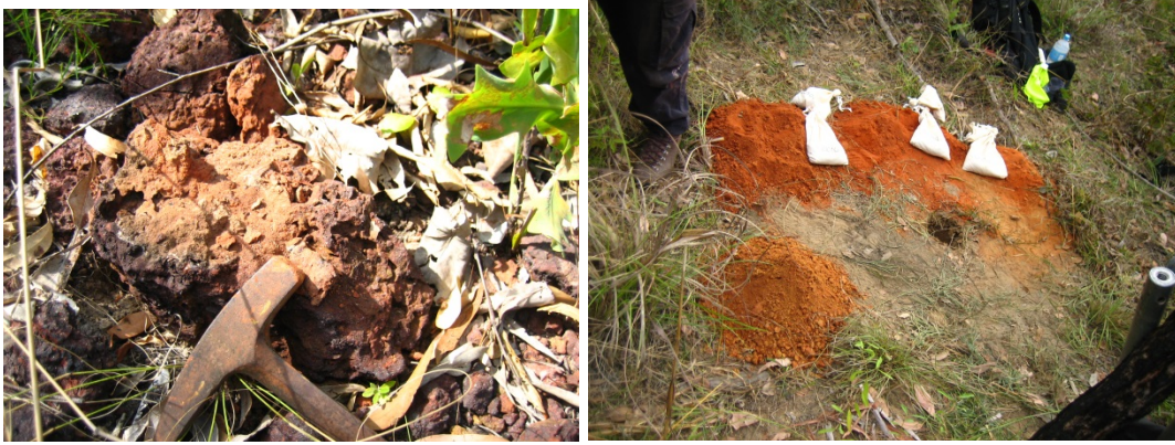
Photo: (left) Typical course, silica rich laterite found in EL 398; (right) deepest hole reaching a depth of 4m, through silica-rich laterite into a saprolite-clay.
