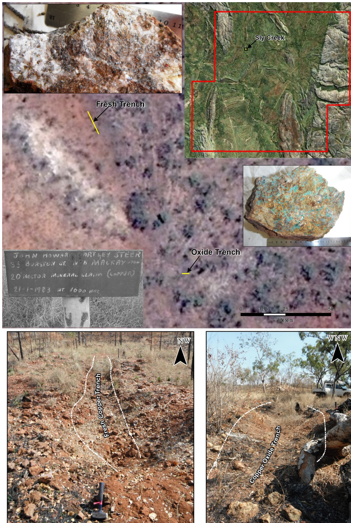
Figure 5: Location of the Sly Creek copper prospect with fresh and oxide copper trenches indicated as yellow lines. Fresh trench mineralisation is dominated by chalcopyrite and the oxide trench is dominated by malachite.
