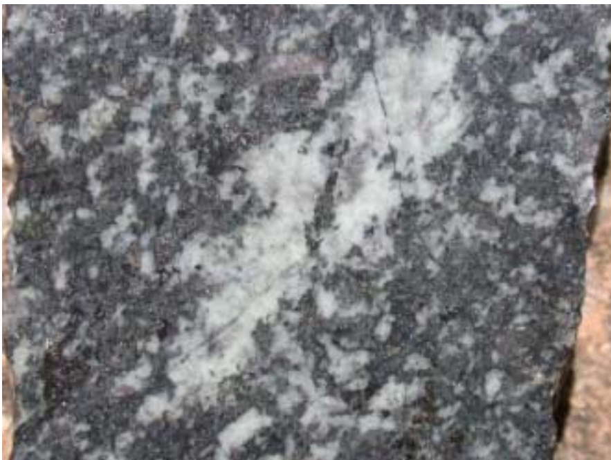
PLATE 1: SAMPLE CX7. Macrophotograph of sawn surface, wet, 4 cm left to right across sample. Note the white feldspar-rich lens which represents a section through primary igneous layering oriented NE-SW.
