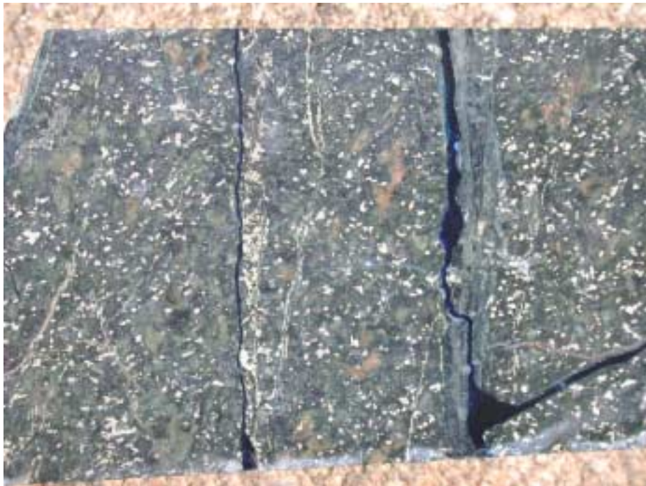
PLATE 2: SAMPLE 01CX6, 21.0m. Sawn drill core, wet, width of core 4.2 cm. Note the thin veinlets and pervasive dull greenish grey altered appearance. Small white disseminated grains are leucoxene/rutile after primary Fe-Ti oxide grains.
