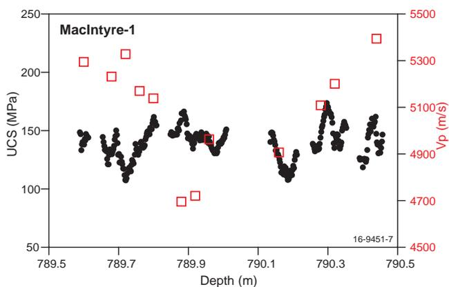
**Figure 3.** Scratch profile of UCS (black dots) and sonic velocity (red squares), obtained on section of drill core from MacIntyre-1 in the Arthur Creek Formation. Over tens of centimetres, large variations in UCS are measured. Gaps in UCS data are associated with breaks or cracks in core (technique requires a 1 cm buffer around cracks for best results).
