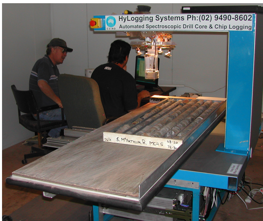
Figure 6. Hylogger machine scanning core during demonstration at Farrell Crescent core facility, October 2008.
