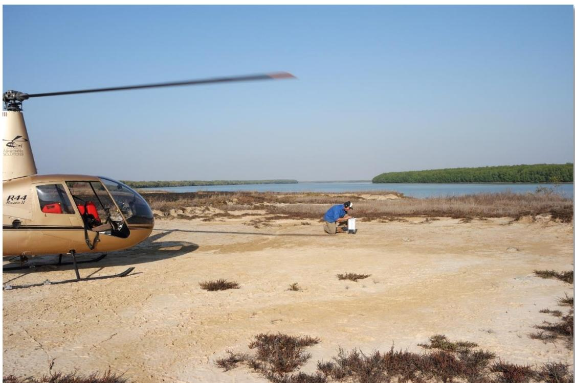
*Photo 1: Gravity reading near the coast*
