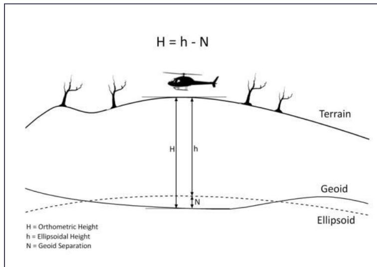
Figure 8: Geoid-Ellipsoid Separation
