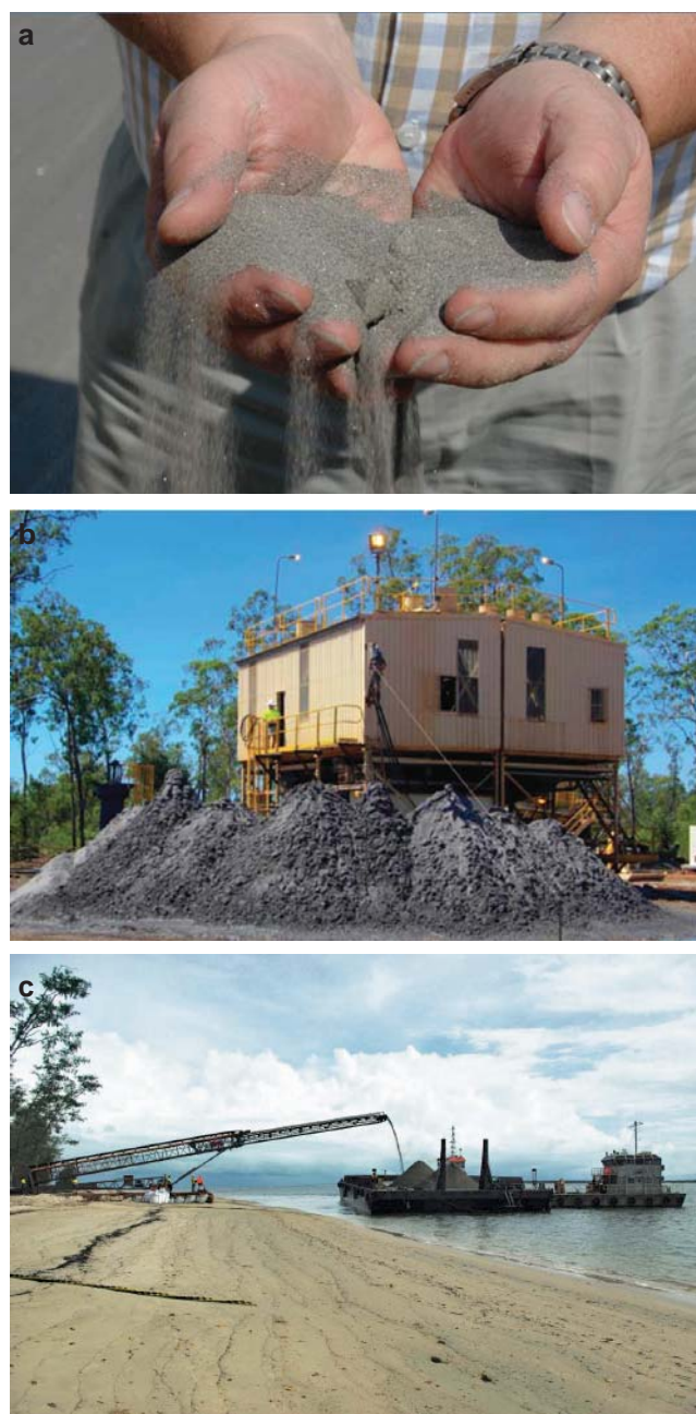
Figure 40.9. Lethbridge heavy mineral sands mining operations (after Matilda Zircon 2011c). (a) Heavy mineral sand concentrate. (b) Lethbridge West processing plant with concentrate stockpile. (c) Conveyor loading heavy mineral sands concentrate onto a barge at Jessie River, Lethbridge Bay, Melville Island.
