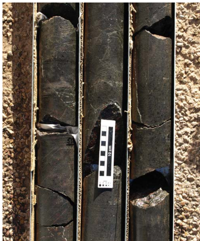
Figure 34.5. Basalt in core from drillhole Hale River-1 at 1694–1697.7 m.
