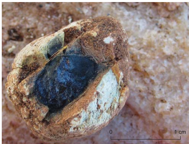
Figure 29.10. Uranium-rich nodule, mainly composed of uraninite, from Yambla uranium prospect, Harts Range (from UXA Resources, ASX Announcement, 5 July 2010).
