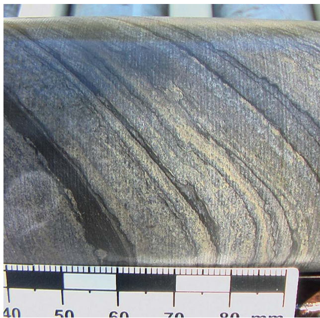
Figure 15.37. Banded sphalerite in drill core from Myrtle prospect (Rox Resources Ltd, drillhole MY16: 189.1 m, 53K 610080mE 8167065mN).
