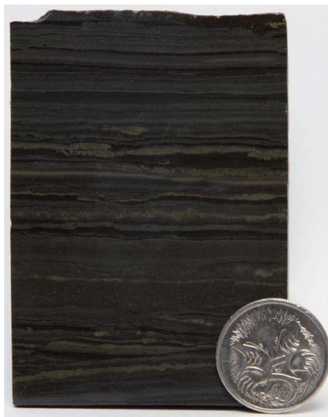
Figure 15.34. Thinly bedded to laminated sphalerite and galena ore typical of the main ore body at McArthur River mine (J Dunster collection).
