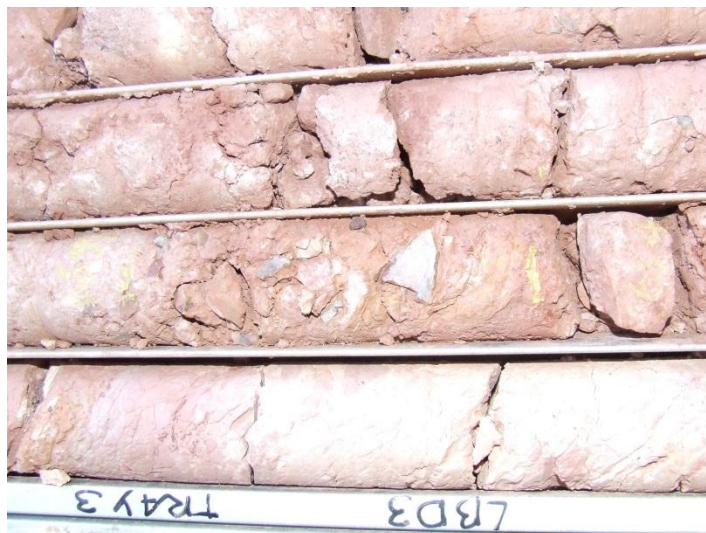
Figure 1 Broken fault Zone
