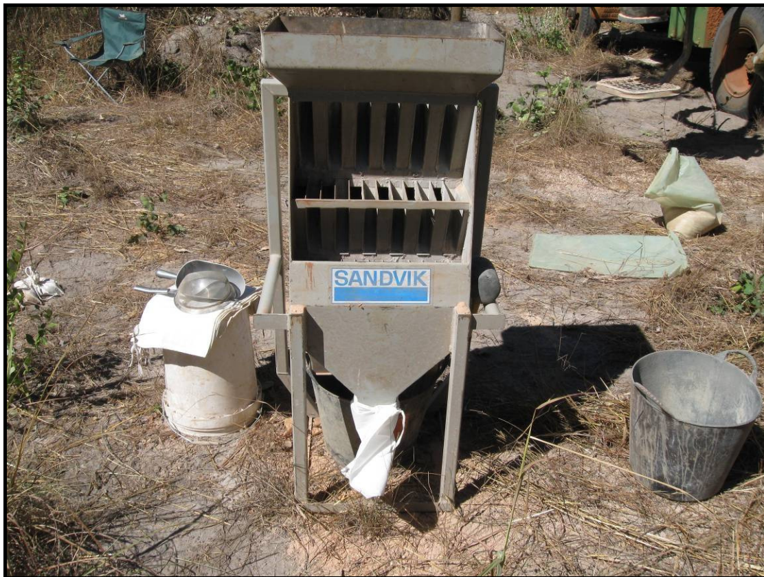
Photo 2: Three-tier splitter used at Bulman
