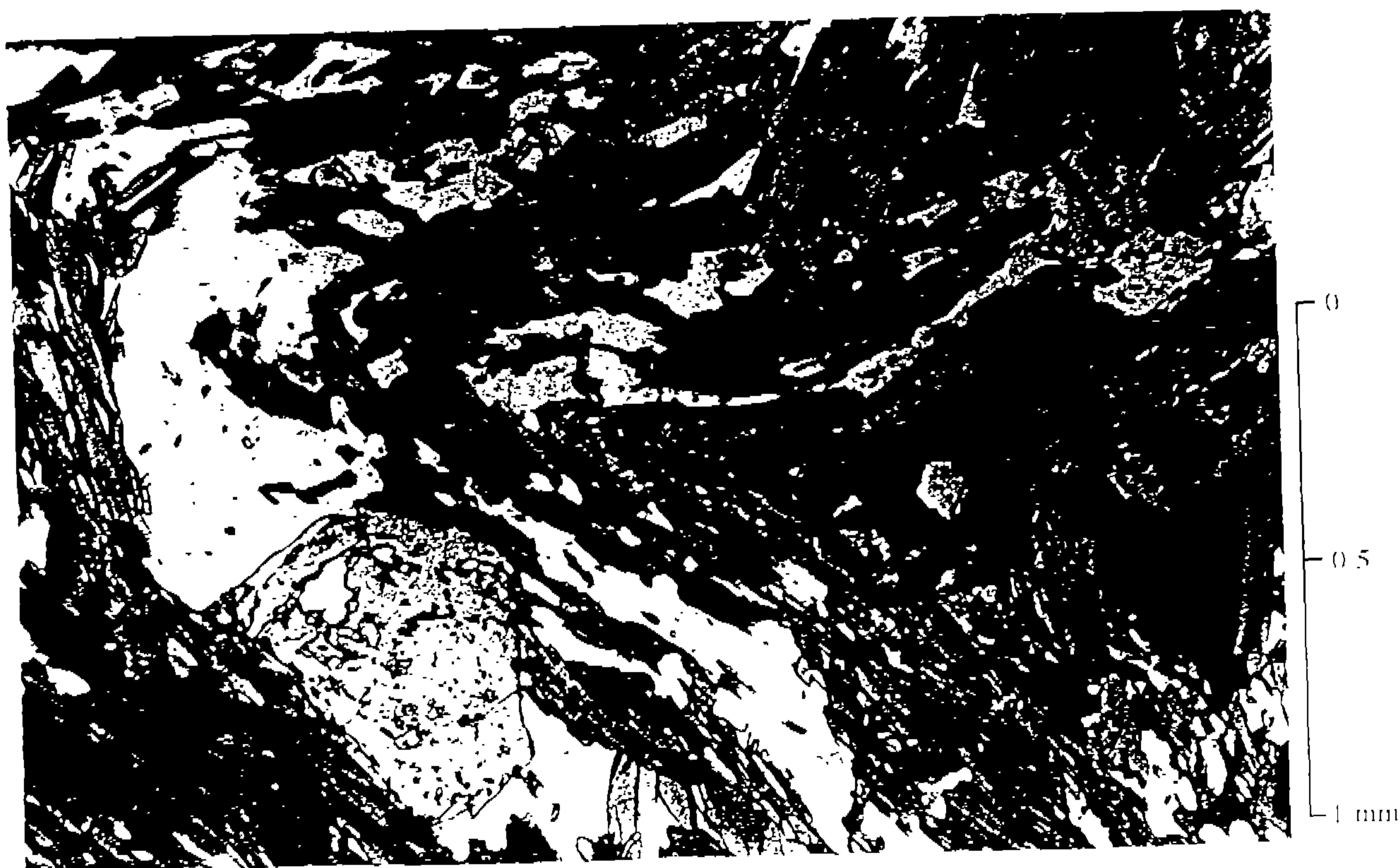
PLATE 2. SAMPLE ALG05, 51 (Transmitted plane polarised light x5 Film 2 Frame 0) In this calc silicate meta sediment, hornblende (green) forms subhedral prisms in a fold structure, accompanied by garnet (equant high relief colourless crystal, lower left) and opaques (black, in fold hinge centre right)
