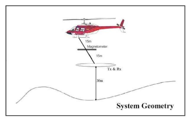
Transmitter loop is towed 30 m below helicopter- Receiver coil is located at centre of Tx loop.
